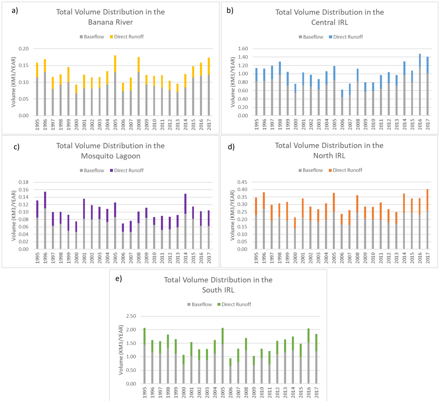
Figure 10. Interannual variation of the baseflow and runoff predicted volumes for each of the IRL Sublagoons: a) Banana River, b) Central IRL, c) Mosquito Lagoon, d) North IRL, and e) South IRL/St. Lucie.
