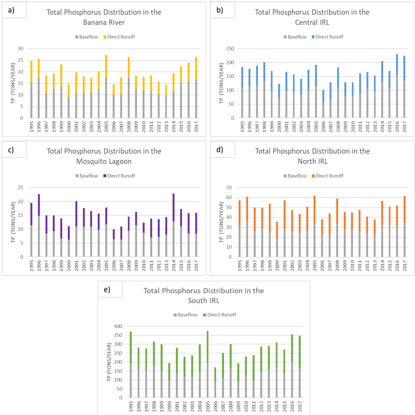
Figure 14. Interannual variation of the baseflow and runoff predicted total phosphorus loading for each of the IRL Sublagoons: a) Banana River, b) Central IRL, c) Mosquito Lagoon, d) North IRL, and e) South IRL.
