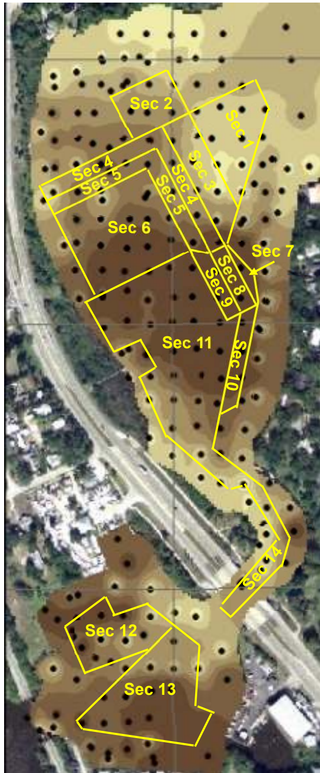
Figure 3.1.2. Contour map of muck thicknesses in Turkey Creek before dredging in February 2015 with overlying dredge cuts SEC-1 to SEC-13 (yellow lines). Image credit for dredge cuts: Brevard County Natural Resources Management Department.
