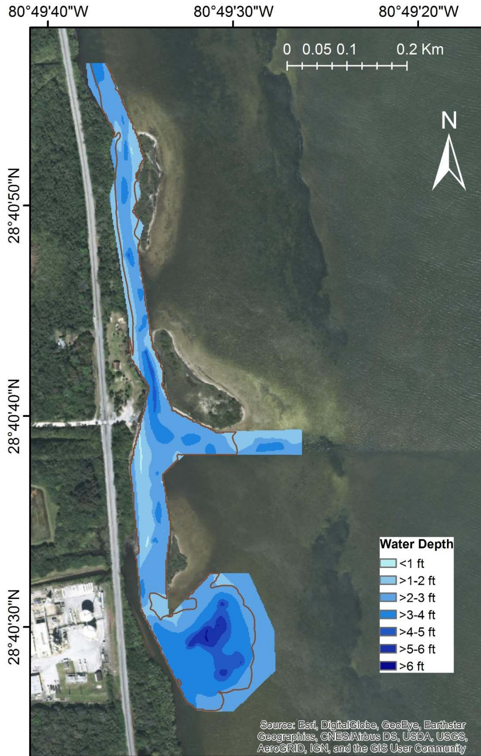
Figure 4.1.2. Contour map of water depth at the Mims Boat Ramp showing water depths prior to dredging.
