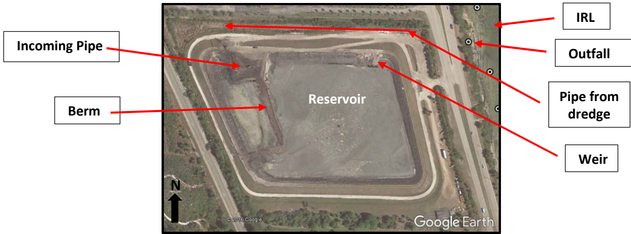
Figure A1. Satellite image of the Palm Bay Dredge Material Management Area (DMMA, BV-52) with arrows and text boxes to identify selected components and the adjacent Indian River Lagoon (IRL).
