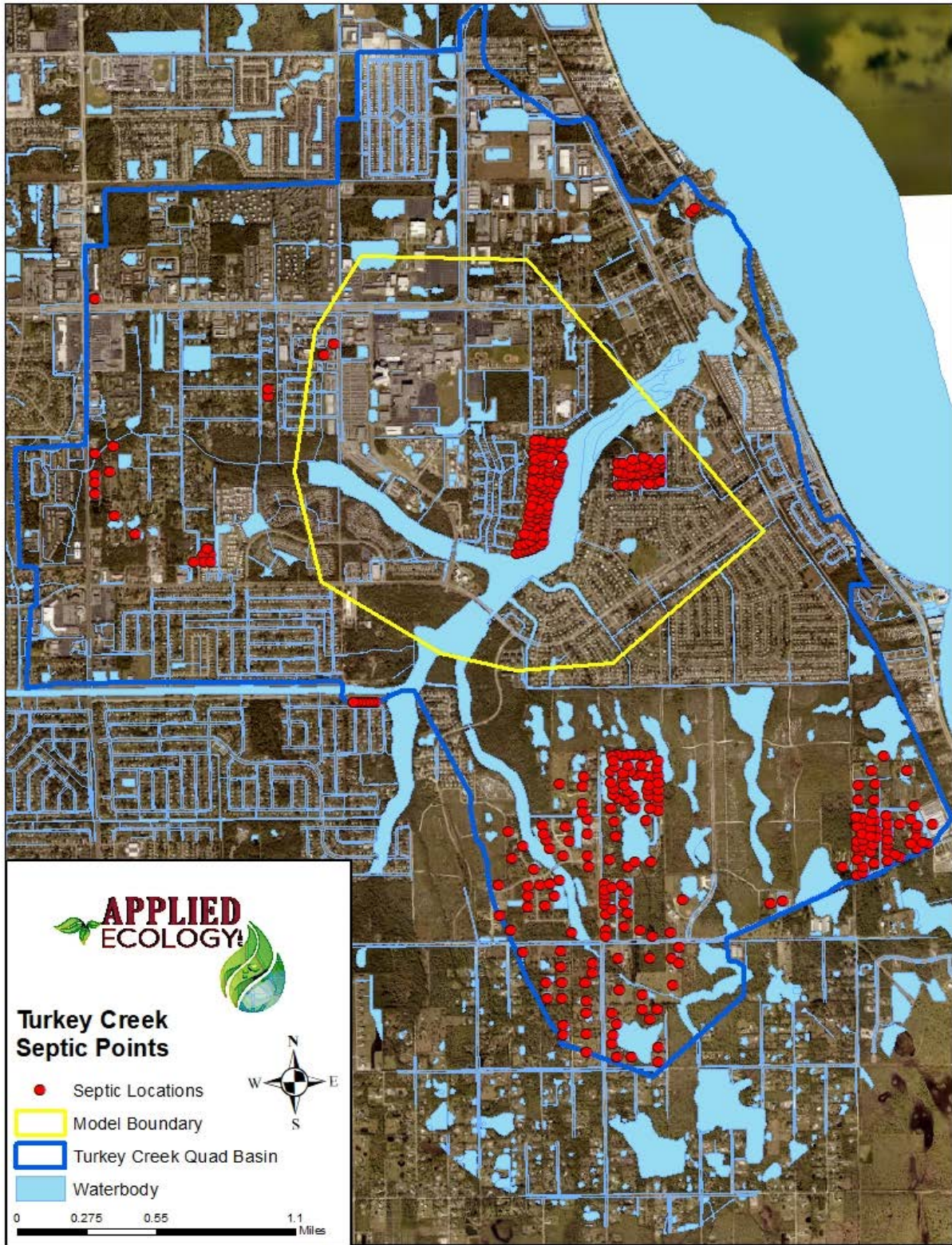
Figure 19: Septic tanks within the Turkey Creek quad-basin that were used in the calibrated run of ArcNLET.
