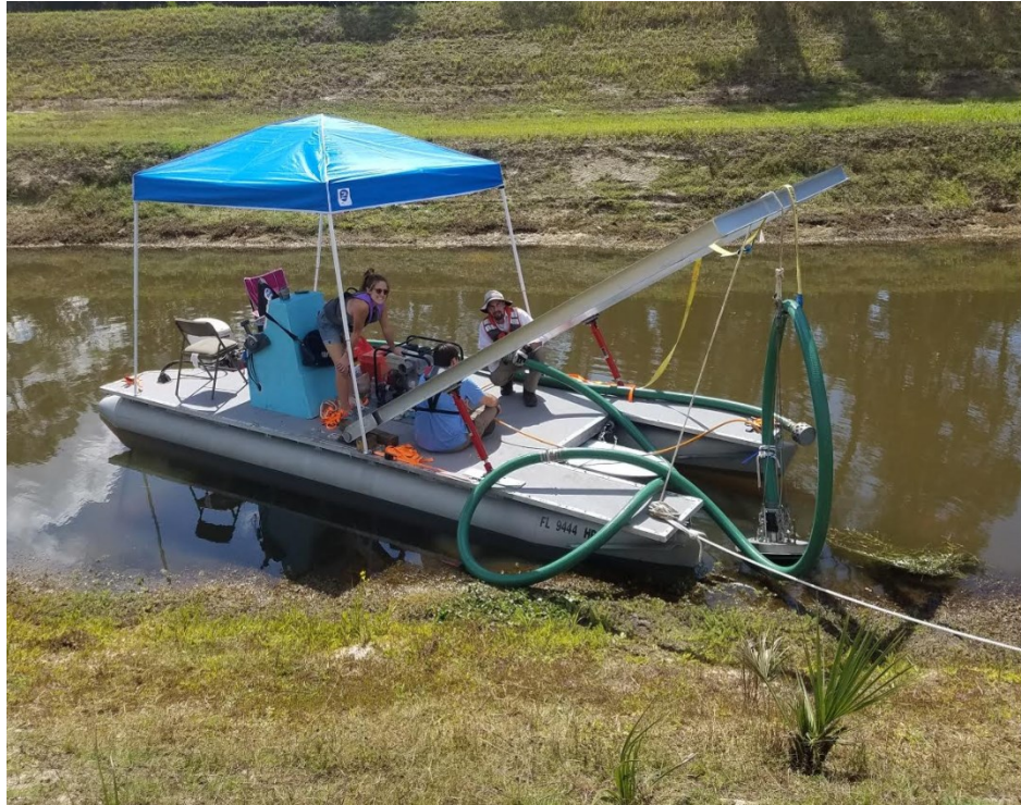
Figure 8: Pontoon Boat with Suction Head Deployed
