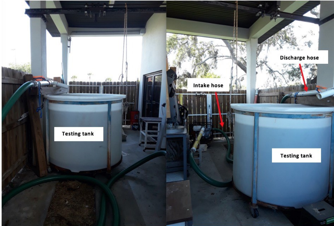
Figure 2: On-campus laboratory setup with testing tank and intake/discharge hoses
