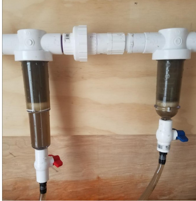
Figure 11: Dredge Slurry Actively Pumped Through Hydrocyclones
