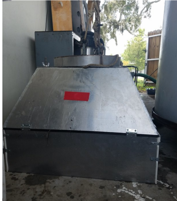
Figure 7: Rectangular Shroud with Extension Attached
