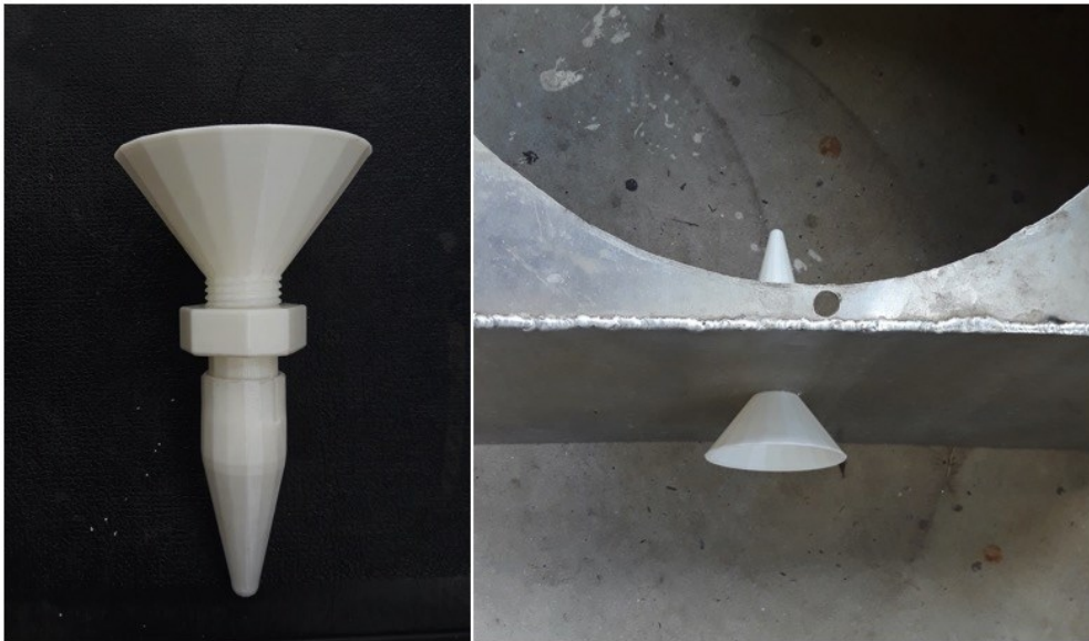
Figure 6: 3D Printed Passive Jet
