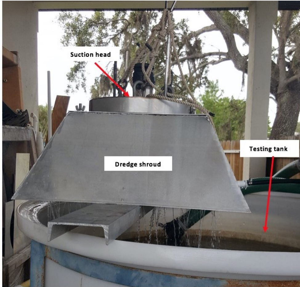
Figure 4: Rectangular Shroud Attached to Suction Head
