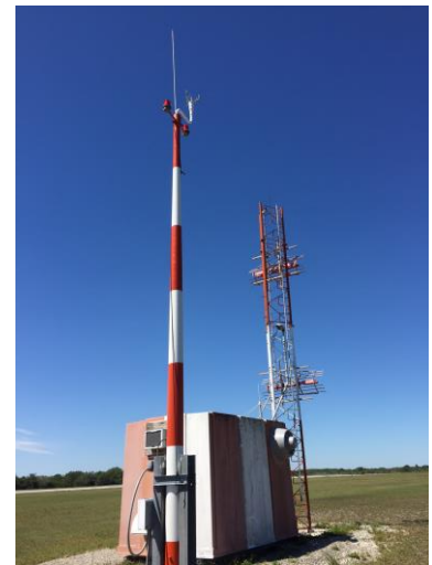
Figure 2.10 View looking west from KFPR. The ultrasonic (glide slope) anemometer is foreground (background).
