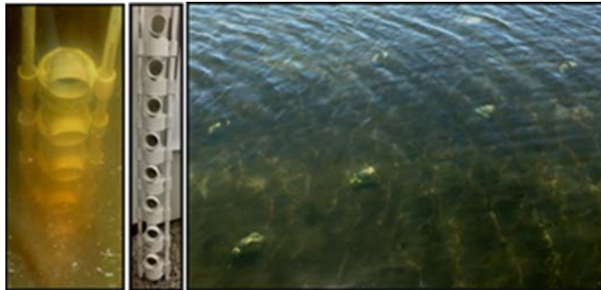
Figure 7. Vertical array of eight horizontal flux sondes in the field (left). The left and the center image shows the array of sondes in the field and lab. Field deployments were conducted August 1 to November 12, 2016. The right image shows the horizontal flux sondes located in a horizontal array (4.5 x 2 m). From Bostater, Rotkiske, Oney and Obot, 2017. Also see the cover of this report for images.
