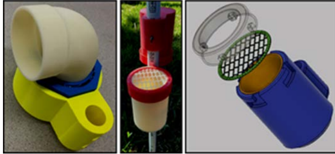
Figure 6. Fluid mud sondes created using 3-D printers based upon computer aided designs originally described in Bostater and Yang, 2014. From Bostater, Rotkiske, Oney and Obot, 2017, and shown on the cover of this report.
