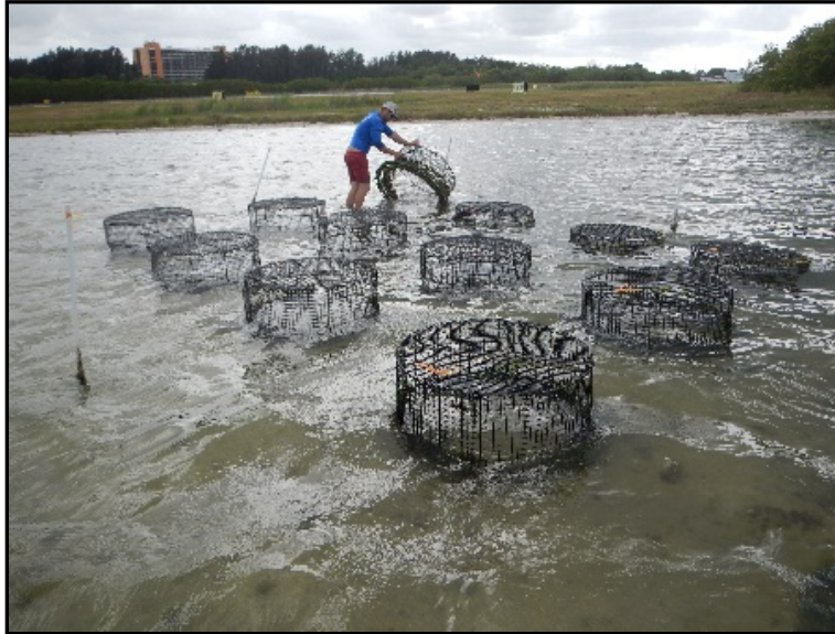
Figure 19. Stainless steel GrowSAV™ Herbivory Exclusion Devices used by Sea and Shoreline, LLC, to protect newly-transplanted seagrasses from large herbivores.
