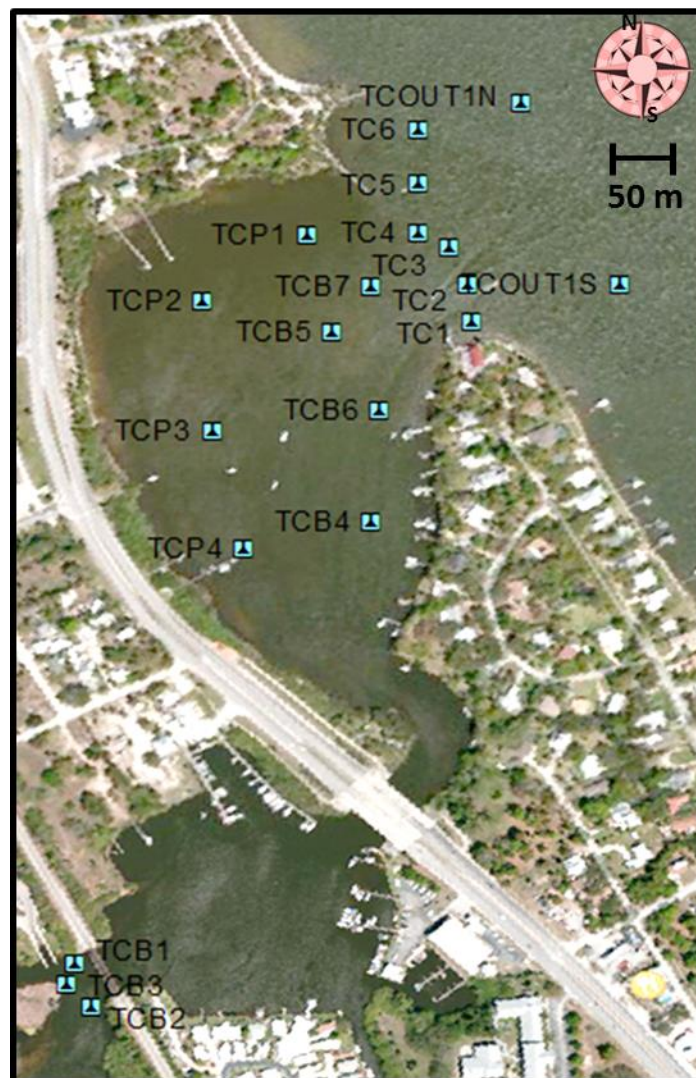
Figure 4.3 Pre-dredge fluidized muck and mud sample locations during 2015. Stations were selected using stratified random sampling in order to insure stations were located (1) west of the railroad bridge, (2) in the main bay of Turkey Creek and (3) near the mouth of Turkey Creek. Georeferenced satellite image courtesy Digital Globe.
