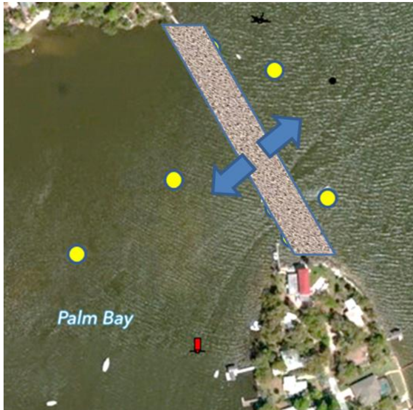
Figure 4.6 Conceptual bottom lutocline and nepheloid layer (0.5 m deep) through which fluid mud and muck movement was measured using the sondes. The horizontal and vertical sonde measurements allow one to extrapolate the mass movement or flux density – lbs. per year moving through an idealized bottom cross-sectional area ( vertical slice ) as depicted above.
