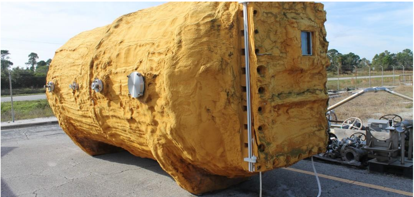
Figure 1: Mars environment chamber wrapped in protective insulation awaiting transport to FIT
