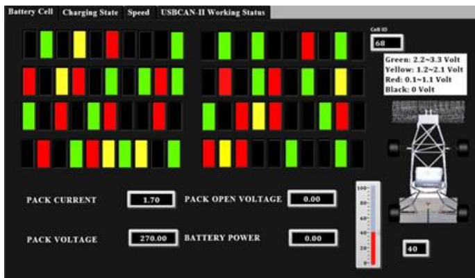
Figure 1: The User Interface using LabVIEW, displaying the states of each of the battery cells in the pack
