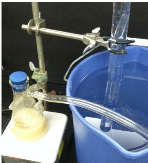
Figure 1: Arrangement for silver nanoparticle-baker's yeast biotoxicity experiment.
