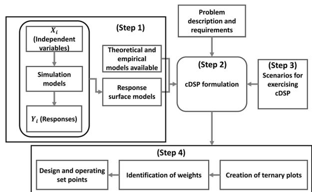
Fig. 2 cDSP-based method to predict set points [22,23]
