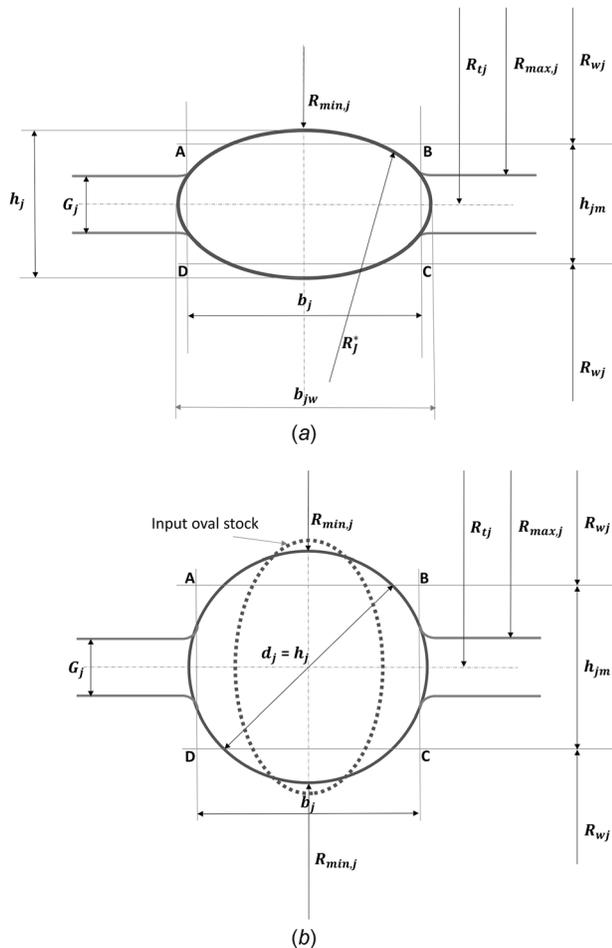
Fig. 4 (a) and (b) Oval and round passed with key dimensions
