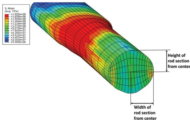
Fig. 6 Cross section of rod produced using FE simulation showing the stress contours and the geometrical variables measured for calculating rod ovality
