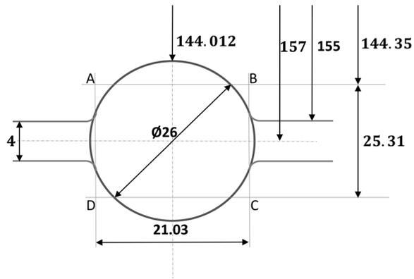
Fig. 18 Pass 4 dimensions designed
