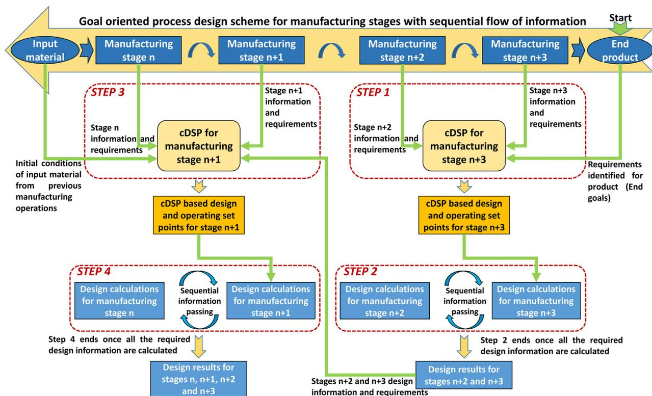
Fig. 3 Goal-oriented, inverse design method for manufacturing stages having sequential flow of information
