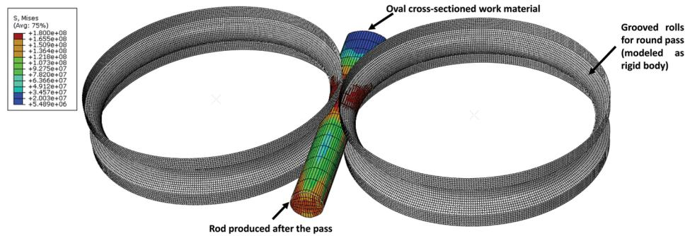
Fig. 5 Geometry and mesh of the FE model developed for rod rolling
