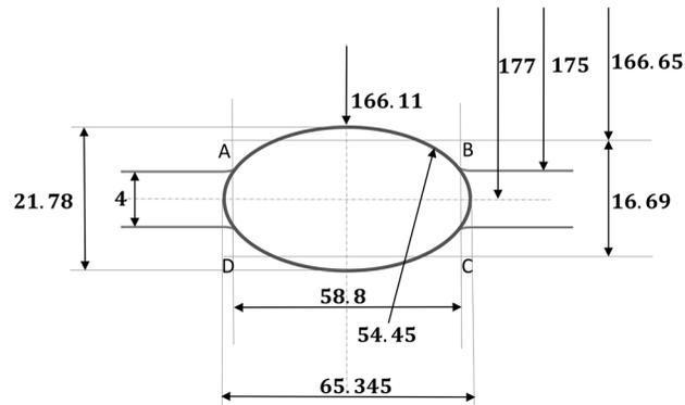
Fig. 15 Pass 1 dimensions designed
