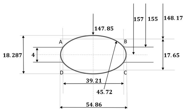
Fig. 17 Pass 3 dimensions designed
