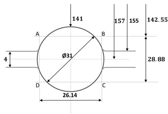
Fig. 16 Pass 2 dimensions designed
