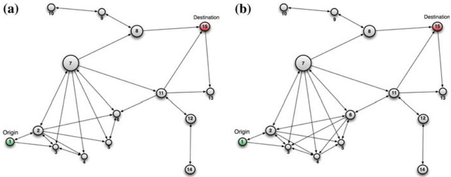
**Fig. 5** Illustrative examples of arc-disjoint and node-disjoint ODDPND solutions. **a** Arc-disjoint ODDPND solution. **b** Node-disjoint ODDPND solution
