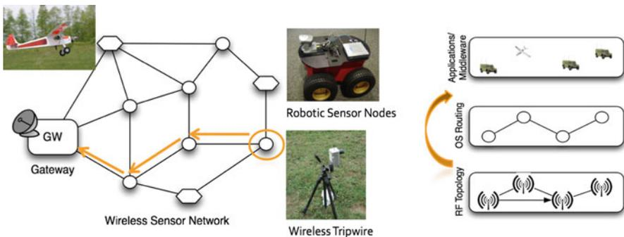
**Fig. 1** Conceptual view of a wireless sensor network and an example of information flow
