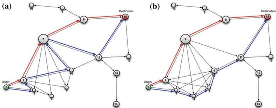
**Fig. 6** Illustration of possible arc-disjoint and node-disjoint dual data paths. **a** Possible arc-disjoint dual data paths. **b** Possible node-disjoint dual data paths
