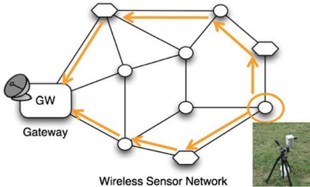
**Fig. 2** Multi-path routing in wireless sensor networks
