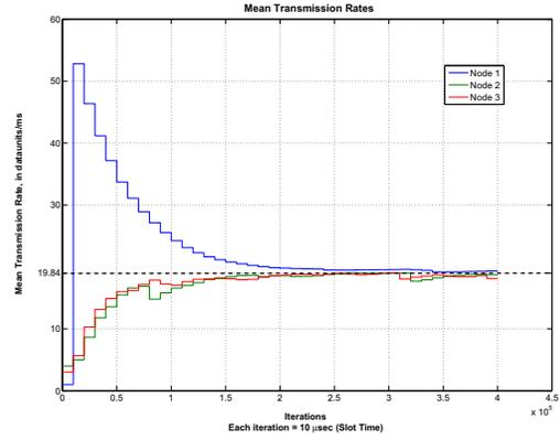
Fig. 3. Mean transmission rates of nodes 1, 2, and 3 transmitting to the same node 4. All nodes are in the sensing region. The online algorithm of (11) is used with  $T = 100 \text{ ms}$ ,  $K = 5$ , and  $\delta T_s = 0.001 \text{ ms}$ .
