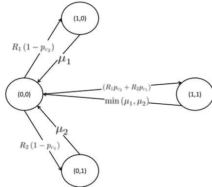
Fig. 2. CSMA Markov chain for a 2-link scenario with collision states.
