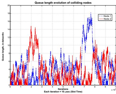
Fig. 4. Queue lengths of nodes 1 and 2 transmitting to the same node 3. The optimum values of the mean transmission rates are the solution to the constrained problem defined in (8), (13), and (14). All nodes are in the sensing region.  $\delta T_s = 0.01$  ms,  $R_1 = 6.05$  dataunits/ms,  $R_2 = 6.49$  dataunits/ms,  $\lambda_1 = 0.16$  dataunits/ms,  $\lambda_2 = 0.2$  dataunits/ms.
