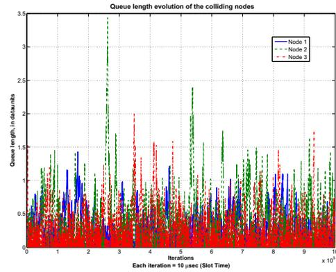
Fig. 5. Queue lengths of nodes 1, 2, and 3 transmitting to the same node 4. The optimum values of the mean transmission rates are the solution to the constrained problem defined in (8), (13), and (14). All nodes are in the sensing region.  $\delta T_s = 0.01$  ms,  $R_1 = 6.54$  dataunits/ms,  $R_2 = 10.19$  dataunits/ms,  $R_3 = 11.49$  dataunits/ms,  $\lambda_1 = 0.02$  dataunits/ms,  $\lambda_2 = 0.05$  dataunits/ms,  $\lambda_3 = 0.05$  dataunits/ms.
