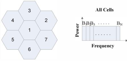
Fig. 1. Reuse-1 scheme deployment. In this scheme all the cells transmit on all available sub-carriers in the spectrum with the same power.
