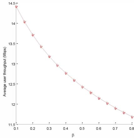
Fig. 8. Average user throughput for SFR with  $\alpha = 0.4$ , and  $\gamma = 0.8$ , as a function of power ratio  $\beta$ .
