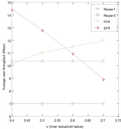
Fig. 5. Average user throughput for Reuse-1, Reuse-3, FFR, and SFR, with  $\gamma = 0.8$ , and SFR power ratio  $\beta = 0.1$  as a function of  $\alpha$
