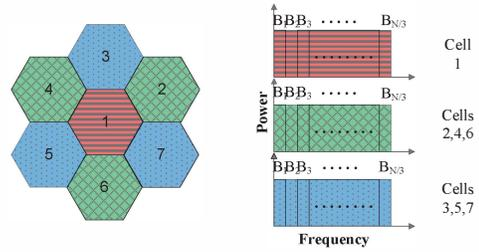
Fig. 2. Reuse-3 scheme. In this scheme no neighboring cells use the same spectrum.
