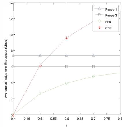
Fig. 7. Average cell-edge user throughput for Reuse-1, Reuse-3, FFR, and SFR, with  $\alpha = 0.4$ , and SFR power ratio  $\beta = 0.1$  as a function of  $\gamma$
