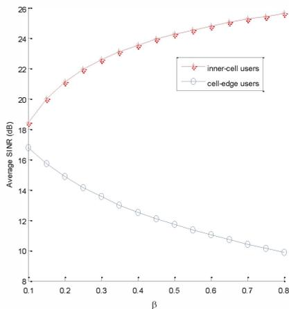
Fig. 9. Average cell-edge, and inner-cell user SINR for SFR with  $\alpha = 0.4$ , and  $\gamma = 0.8$ , as a function of power ratio  $\beta$ .
