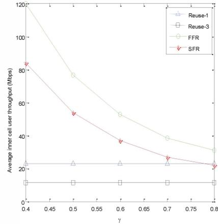
Fig. 6. Average inner cell user throughput for Reuse-1, Reuse-3, FFR, and SFR, with  $\alpha = 0.4$ , and SFR power ratio  $\beta = 0.1$  as a function of  $\gamma$
