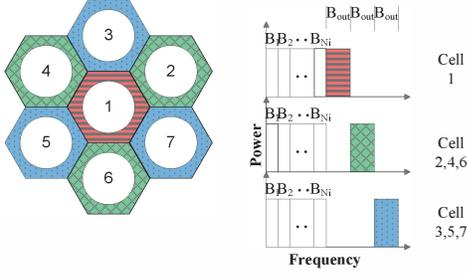
Fig. 3. FFR scheme. In FFR, the reuse factor for interior users is 1 and the reuse factor for exterior users is 3.
