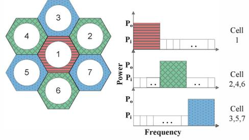
Fig. 4. SFR scheme. In this scheme inner RBs transmit with a higher transmit power than RBs used for cell-edge users.
