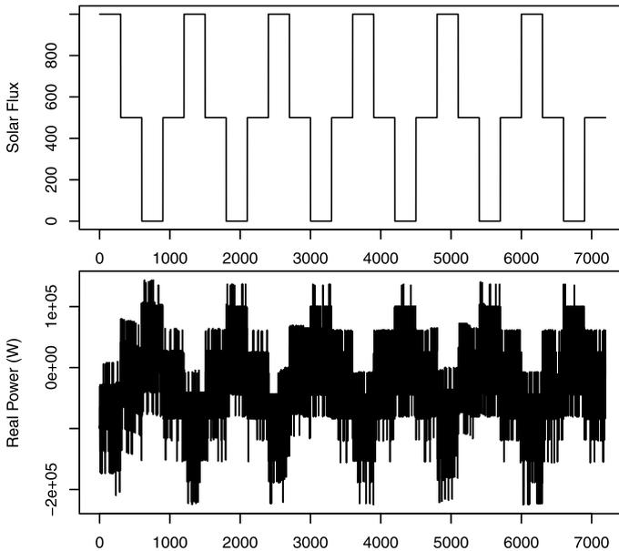
**Fig. 6** Effect of a variable communications delay (top level meters have a communications delay between 10 and 30 ms, and the batteries and their respective meters have communication delays between 70 and 100 ms). The agent update rate is 100 ms
