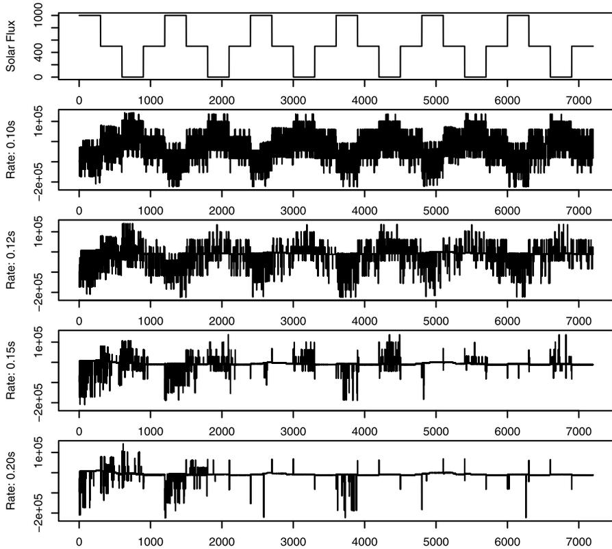
**Fig. 7** Result of compensating for the variable communications delay using different update rates
