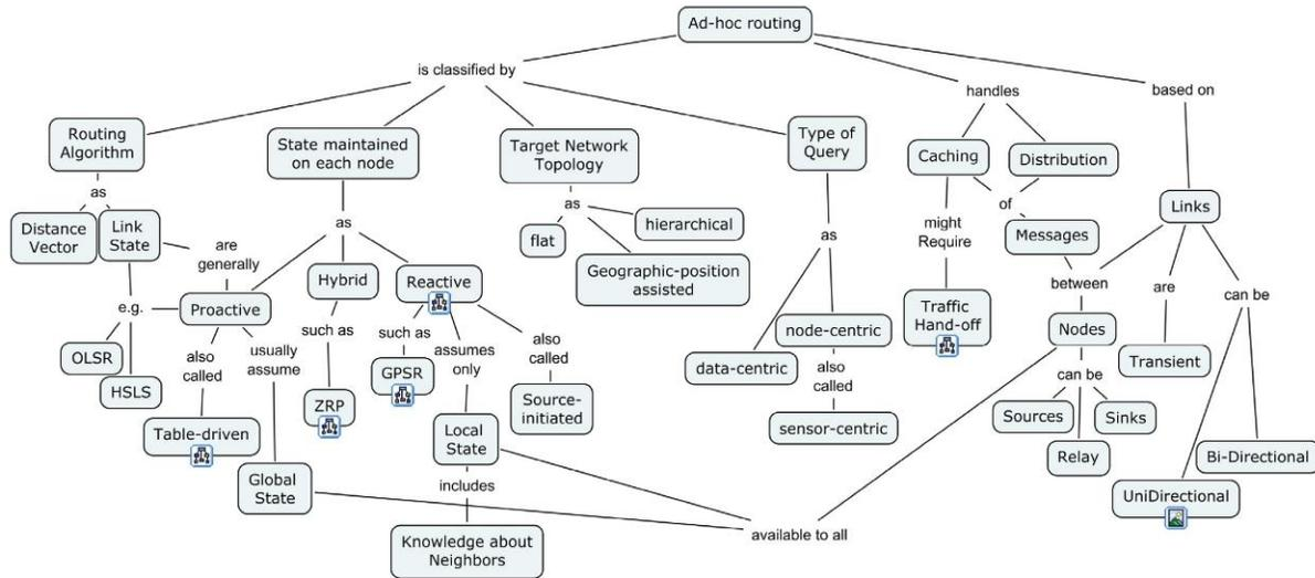
Figure 1. Classes of ad hoc routing protocols.
