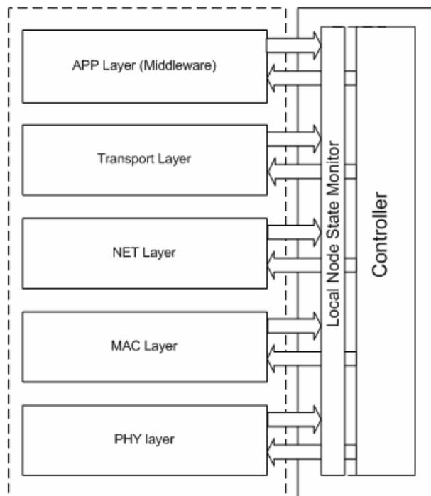
Figure 1. Cross-layer integration through a common controller component
