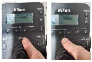
To move the sample slide up and down in Z axes to get the sample in a focus plane use the focus knob on the manual pad or on the microscope. Similar to the previous step if you press button the movement will be faster.
