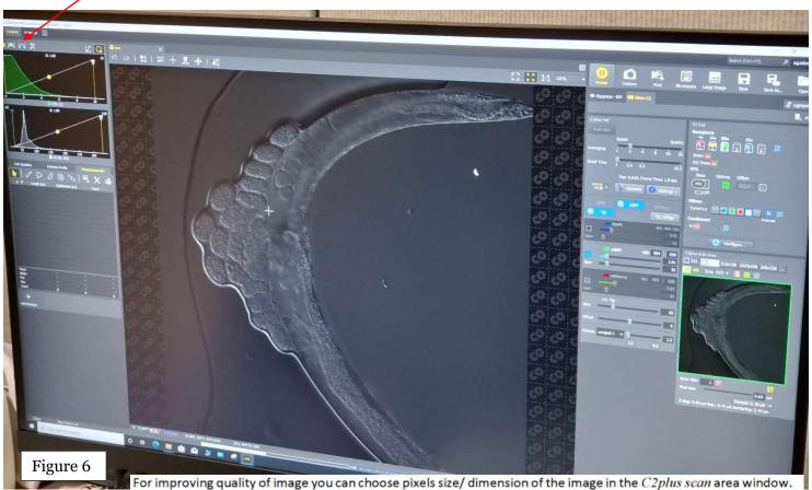
"1024" is acceptable dimension for capturing the image. The bigger the dimension the longer the capturing time will proceed.
