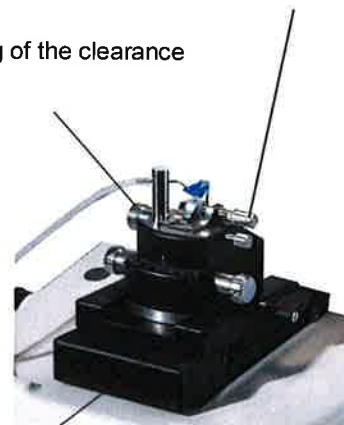
Precision drive for pivoting the knife.
