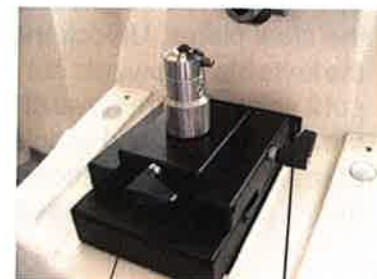
Clamping lever of the trimming block
