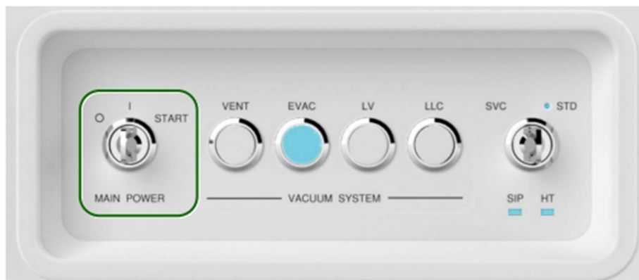
Fig.9. Main control panel on the electron column unit shows that EVAC button is lit with blue color - Sample chamber is under the vacuum.
