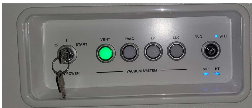
Fig.10. VENT button is lit with green and not blinking – the sample chamber is at atmospheric pressure.
