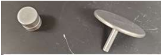
Sample stubs; specimens are mounted onto them using double sided carbon adhesive tabs
