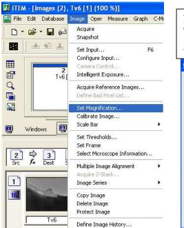
Next set the magnification, Image > Set Magnification. This step must be done in order for the next step to give you the correct scale bar.
