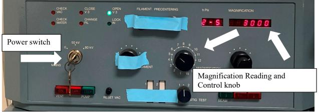
Turn the power on to the TEM by turning the key switch to 50kV or 80kV (50kV is used for most biological applications); check that the magnification is set at 3000X. Note: If there is blue tape over the top of something, this is something you should not change.
