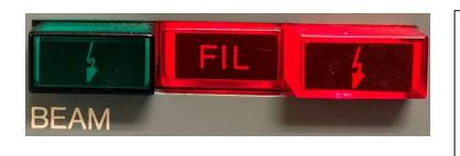
Now the green button on the left will go out and the red button on the right will illuminate. Press the center, FIL, button.
