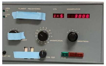
Once V3 is open the green light on Beam button will illuminate. On the right panel depress the  $\mu$ A button and keep depressed while you press the green BEAM button on the left. Watch the Exposure Time gauge to see that the red pin pegs to the right. This confirms that there is power going to the filament.
