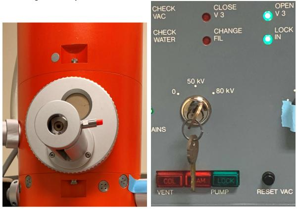
At this point the V3 light should remain illuminated. If for any reason it has turned off press RESET VAC again and wait for it to come back on.
