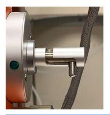
Open V3 by sliding the lever down and then to the right. Make sure it locks into the notch at the end.
