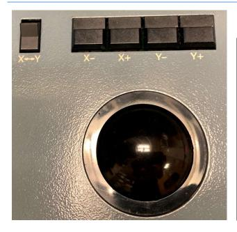
Once you have your sample on the screen you can used the world's hardest to use trackball to move around on your sample. If while moving, your sample it does not go the direction you wish you can push the  $X \leftarrow \rightarrow Y$  button to help it move in the correct direction. While the X-, X+, Y-, Y+ buttons above the trackball will move in the direction you want to go, the movements are too great to be of much help.
