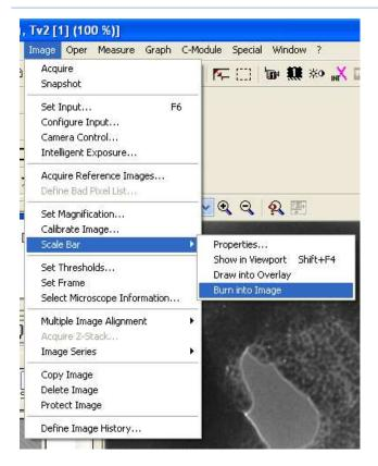
Next burn the scale bar into the Image. Image > Scale Bar > Burn into Image.
