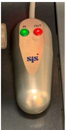
Once you have your sample image in the center of the screen, press the green IN button on the camera control. This inserts the camera under the beam.
