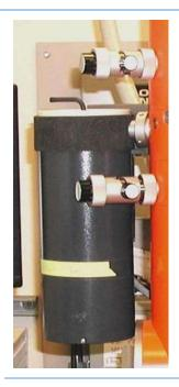
Fill the anti-contamination device, on the left side of the column, with liquid nitrogen. Pour slowly as it will boil off quickly at first and you will need to refill it if it is not filled to near the top. A full device of liquid nitrogen should last for 4 hours. Please see microscopy center manager or approved representative for help in filling it.
