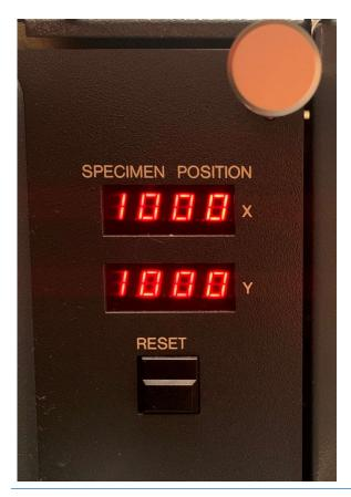
At some point you may end up moving the sample too far to the right, left, top, or bottom and you cannot move your sample any longer. To correct this you must press reset and the sample will reset to the center of the grid.
