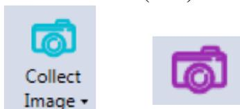
Clicking on the down arrow selection (on the image icon) will display the **Image Collection Parameters** pop up window, shown below. There are three sizes for image collection matrices: 512 x 400, 1024 x 800 and 2048 x 1600 pixels. The larger the values of the matrix, the higher resolution. The selected resolution will appear highlighted on the window.
