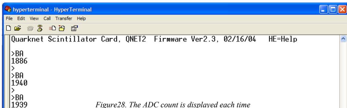
Figure28. The ADC count is displayed each time the ‘BA’ command is typed.
