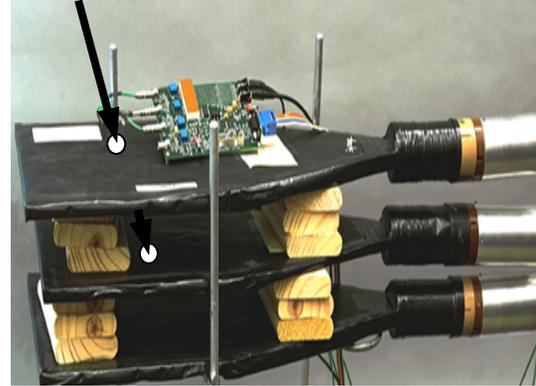
Figure 20. A three counter muon lifetime detector system.
