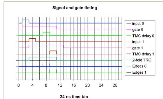
Figure 34. Signal and gate timing diagram for Example A.
