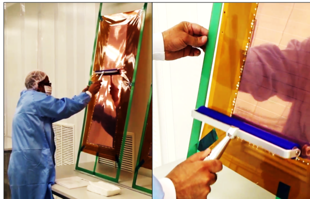
Figure 41: Cleaning of the first side with the static roller.
