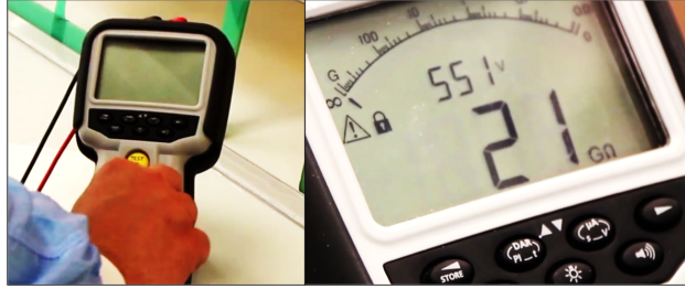
Figure 45: Testing the GEM foil.
