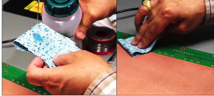
Figure 17: Cleaning of the HV circuit.
