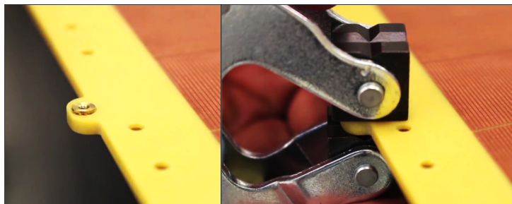
Figure 4: Clamping of the brass inserts.
