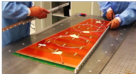
Figure 113: Removing the assembly jig.
