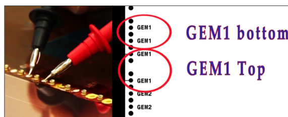
Figure 61: Connecting the insulation meter to the GEM1 pads.
