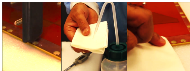
Figure 7: Cleaning of the gas in/outlets.
