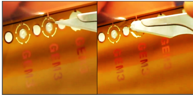
Figure 46: Cutting off the spare HV pads.
