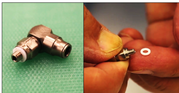
Figure 10: Removing the O-ring from the gas connector.
