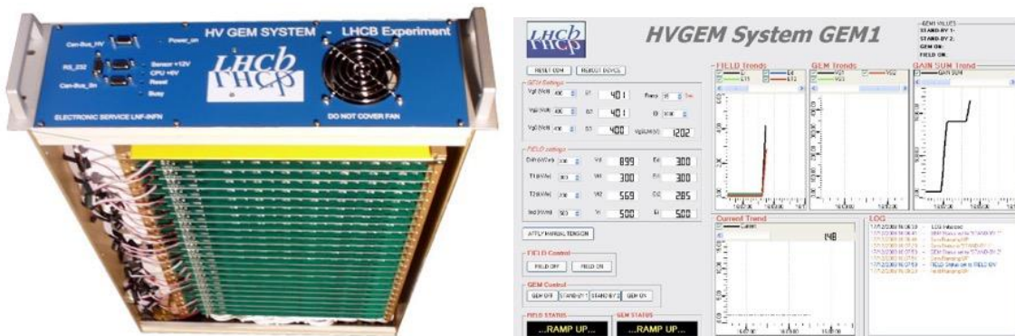
Figure 3.12: LHCb High-Voltage System with 24 HVGEM modules and nano ammeter; on the left the current and voltage monitoring system developed by LHCb.
