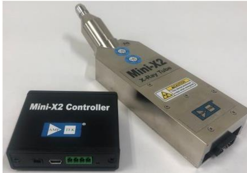
Figure 4.25: The Mini-X2 X-Ray generator by AMPTEK.
