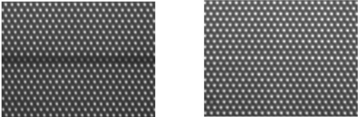
Figure 9.6: Photons emission image recorded with a GEM foil in two configurations of the sectors separation (Marques et al. , 2020).
