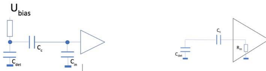
, Figure 8.10 Left: AC-signal coupling for DC-biased detector electrodes. Right: input time constant C_c * R_{in} .
