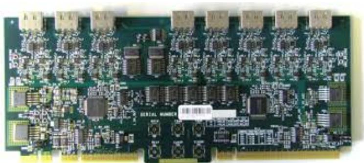
Figure 3.5: SRS Analog-Digital Converter card [20].
