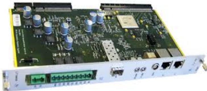
Figure 3.6: SRS Analog-Digital Converter card [20].
