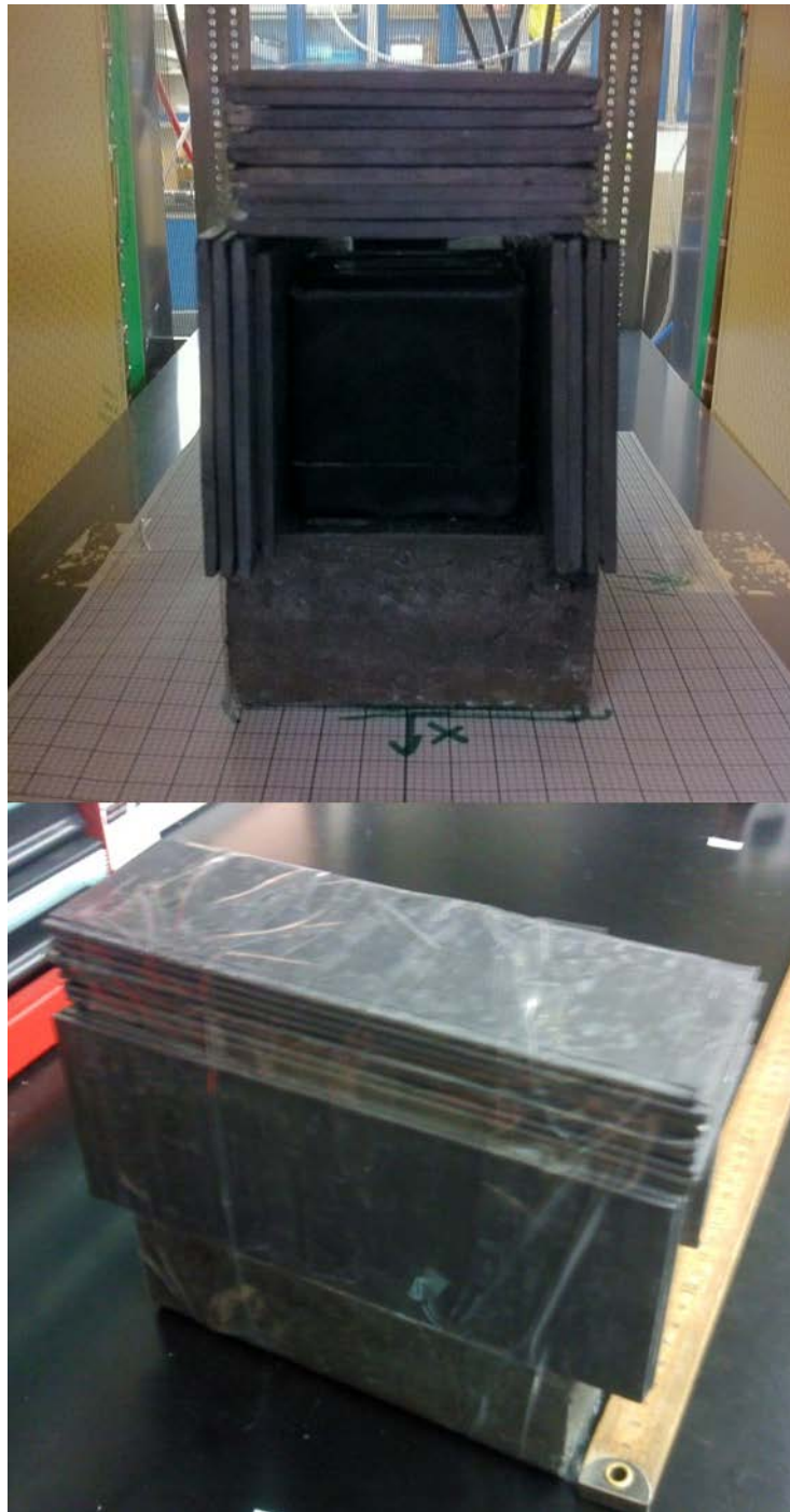
Figure 5.17 Photos of the scenario with strong lead shielding. The 75 \text{ cm}^3 depleted uranium block is placed in the central region and is heavily shielded on all sides.
