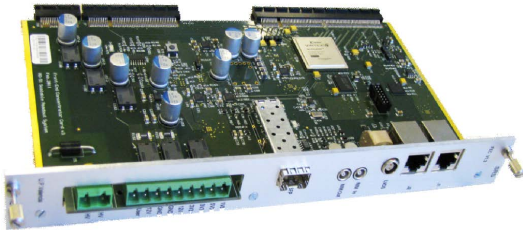
Figure 3.4 The SRS Front-End Concentrator card [26].
