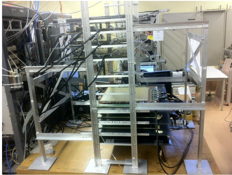
Figure 2.19: Partially loaded MTS prototype II at CERN. Top and bottom detector stacks are fully loaded, but side detectors have not been mounted yet. A target plate with material to be imaged is also missing.
