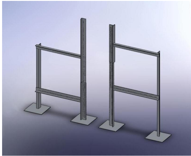
Figure 2.15: Quadrants one and two of our MTS prototype II imaging station. Quadrant two is composed of the same fundamental elements as quadrant one, and they are arranged to accommodate the geometry shown in figure 2.11. In a similar fashion, quadrants three and four are constructed.
