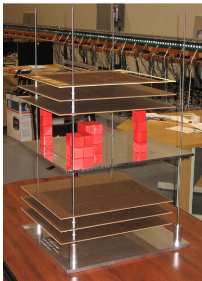
Figure 2.6: MTS prototype I with mock readouts and imaging material from another perspective. The readout at the top of the top stack was an actual readout that had been damaged. One can see the fourth support rod going through the target plate only.
