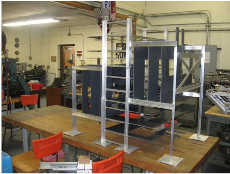
Figure 2.17: Assembled MTS prototype II in Florida Tech's machine shop shortly after its construction was completed in June 2010. The station is loaded with PVC support plates that will be used to secure GEM detectors and scintillators, along with their supporting electronics.
