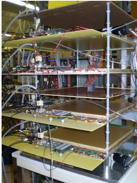
Figure 2.7: Fully commissioned MTS prototype I collecting data at CERN. Note that two GEM detectors are being used in each detector stack, and a small block of lead is being imaged. The damaged readout is able to serve as the target plate here used to image material [23].
