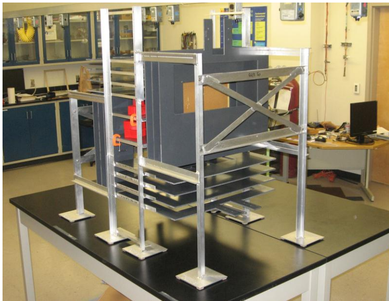
Figure 2.18: Assembled MTS prototype II in Florida Tech's High Energy Physics Lab A. Along with PVC support plates, the station is also loaded with target plates secured by C-clamps and mock material to be imaged.
