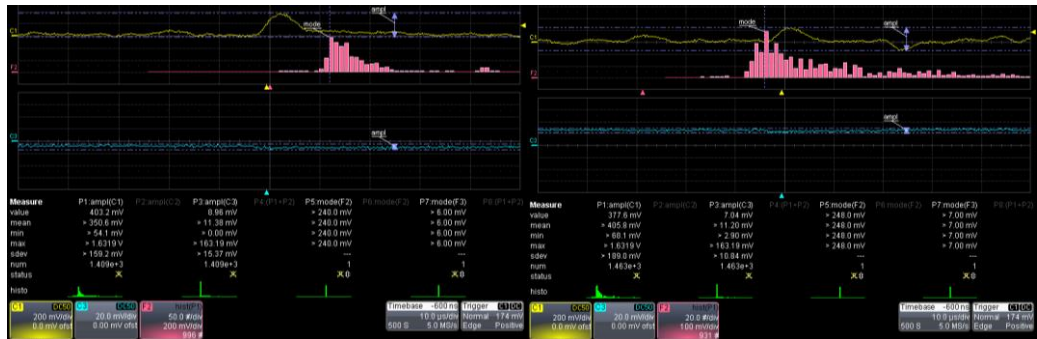
Figure 87: Scope shots of the signal through the pre-amp and amplifier (C1, yellow) and through just the pre-amp (C3, cyan). Histograms of the amplitudes of C1 shown at the beginning of the two-day study (left) and at the end of the two-day study (right), negative polarity
