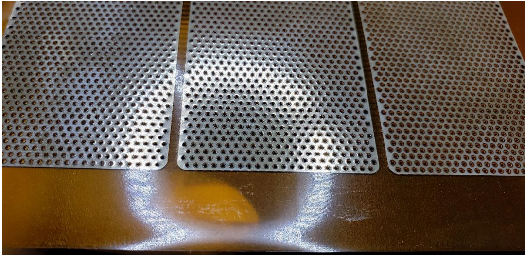
Figure 22: Close-up of three sectors with rim sizes (from left to right) of 0.1mm, 0.15mm, and 0.2mm.
