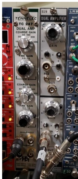
Figure 47: Former amplifier (Tennelec TC 247) on the left, new one (Mech-Tronics Nuclear 519) on the right
