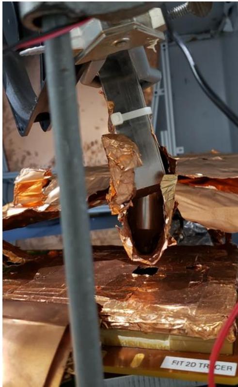
Figure 54: X-ray gun with copper foil filter pointed down at detector.
