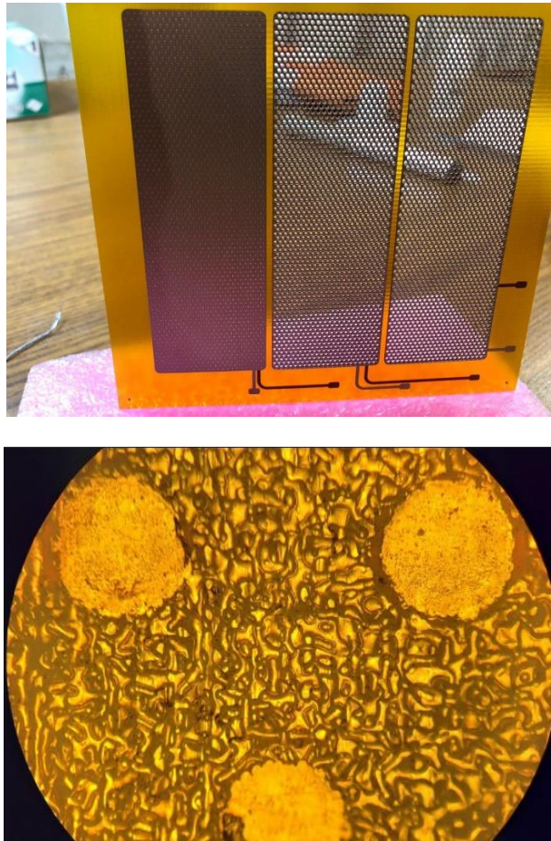
Figure 16: Room light as observed through the THGEM (top). Total clogging of no rim holes with insulating material (bottom).
