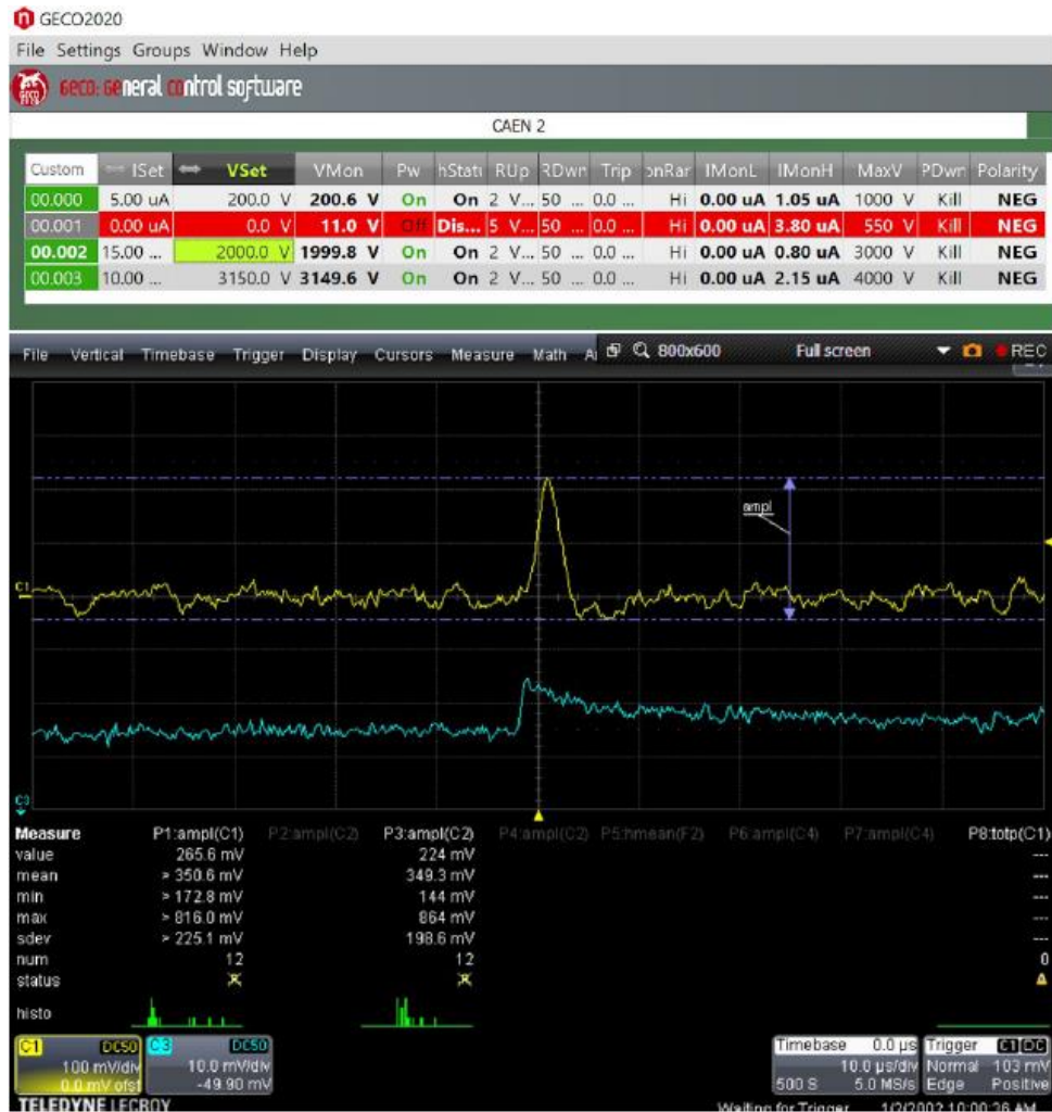
Figure 42: GECO2020 HV Monitoring software (top) and scope traces (bottom) under Fe-55. The top scope trace is through the pre-amplifier followed by the amplifier, and the bottom trace is through only the pre-amplifier. In the GECO2020 software, from top to bottom, the electrodes shown are: THGEM Bottom, (Unused Channel), THGEM Top, Drift.
