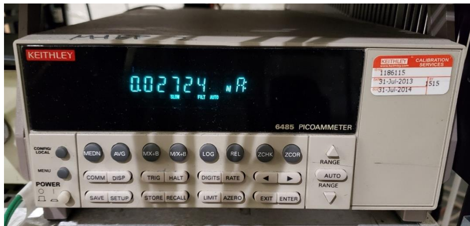
Figure 89: Keithley Picoammeter used for signal current measurements
