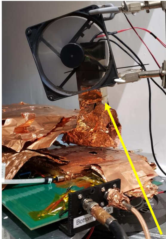
Figure 53: Gain testing setup within a lead-lined X-ray Box. Arrow indicates the X-ray gun. The purpose of the fan is to keep the X-ray gun cool and maintain operating temperature.
