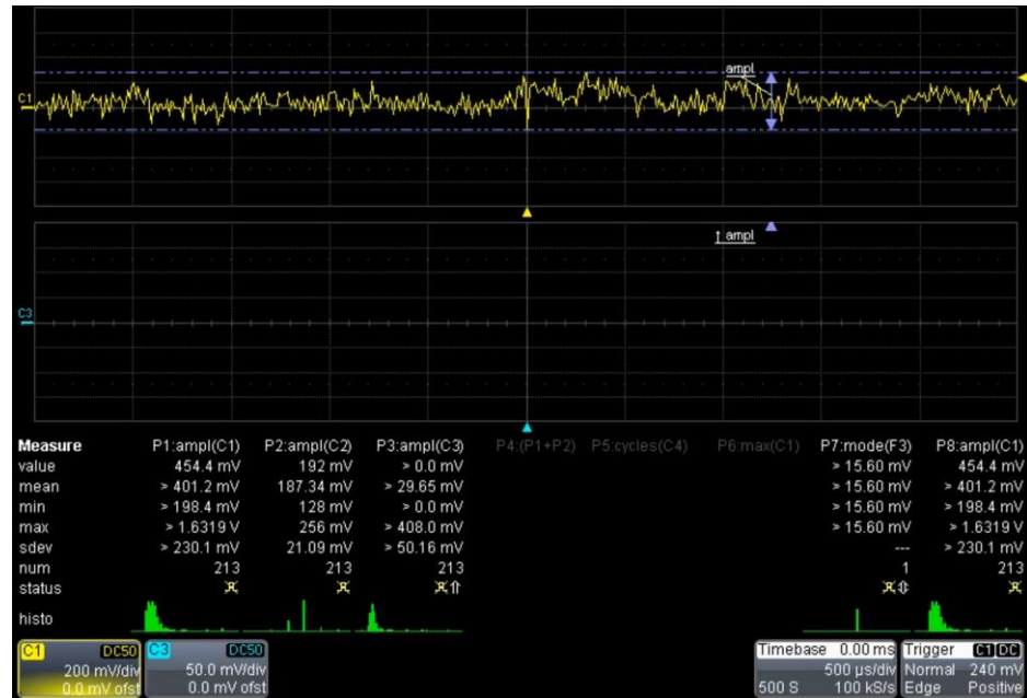
Figure 43: Scope images showing occurrences of some of the various forms of suspected discharges
