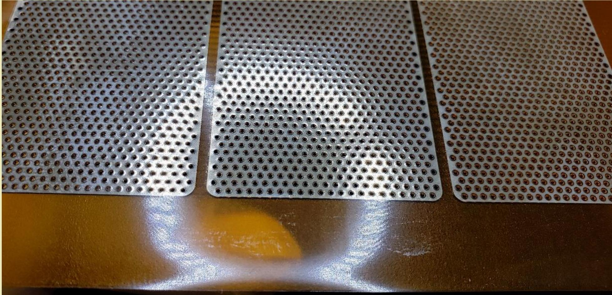
Close-up of the three sectors with rim sizes (from left to right) of 0.1mm, 0.15mm, and 0.2mm.
