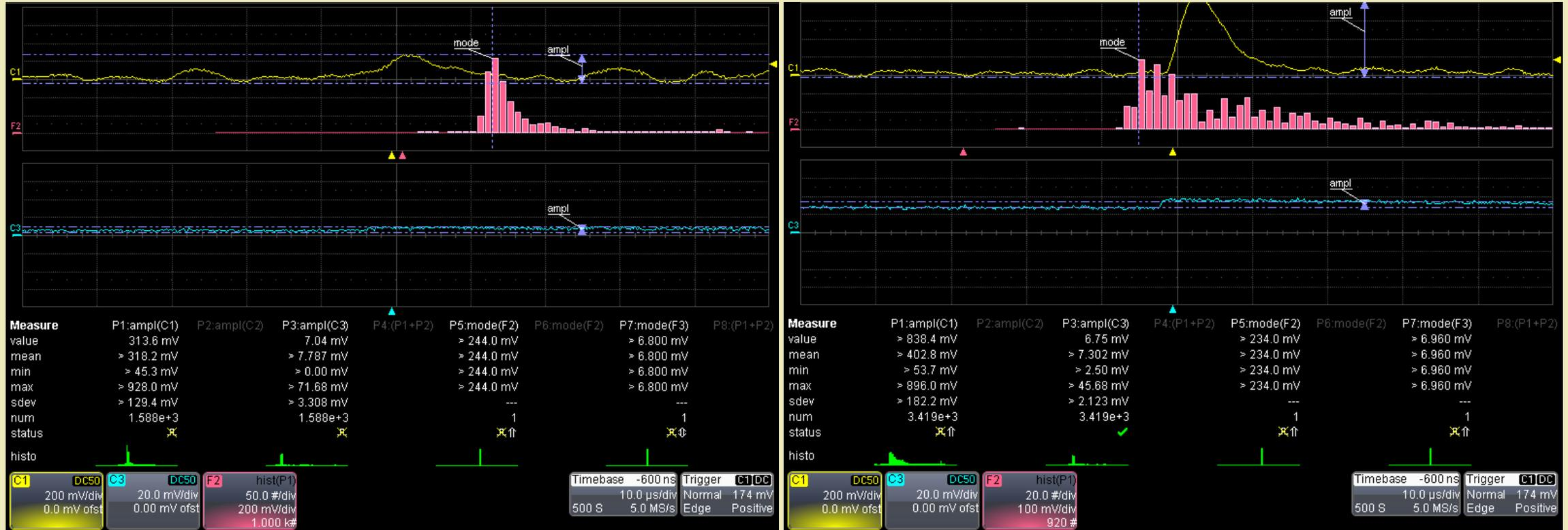
Histogram with amp signal at beginning (left) and end (right) of 48-hour study, positive polarity
