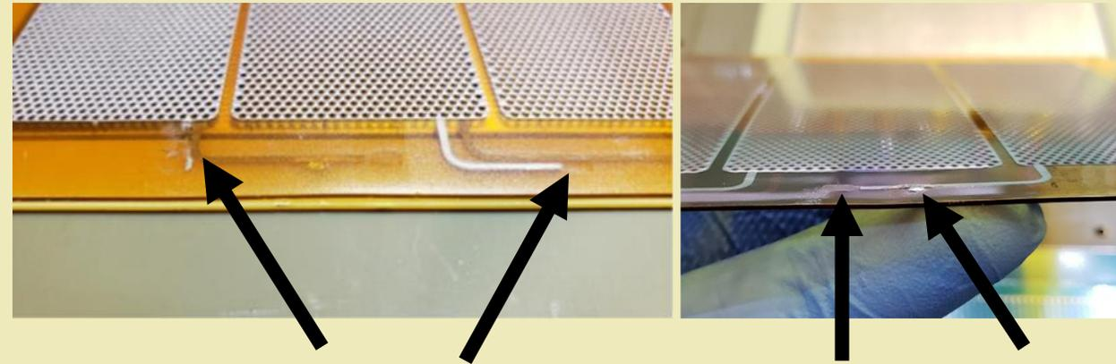
Various damages which can occur through soldering
