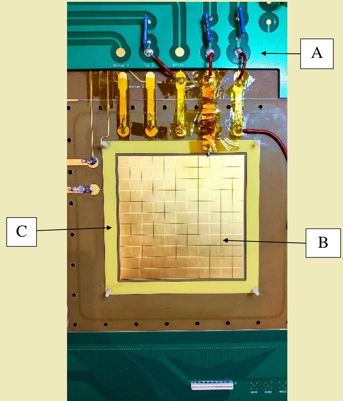
*HV board (A), anode (B), and induction gap spacer (C)*
