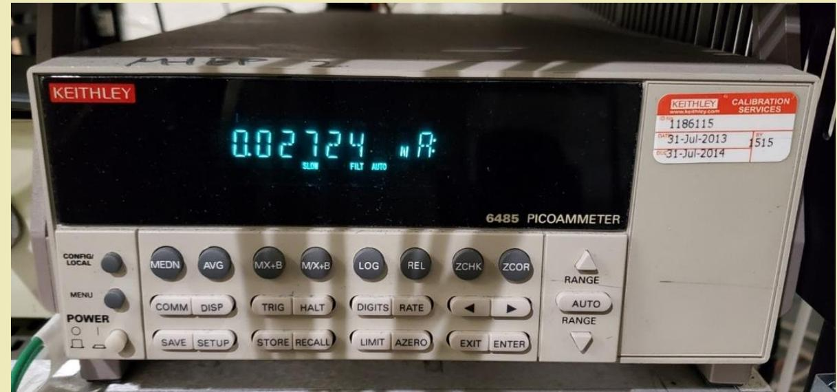
Keithley Picoammeter used for signal current measurements
