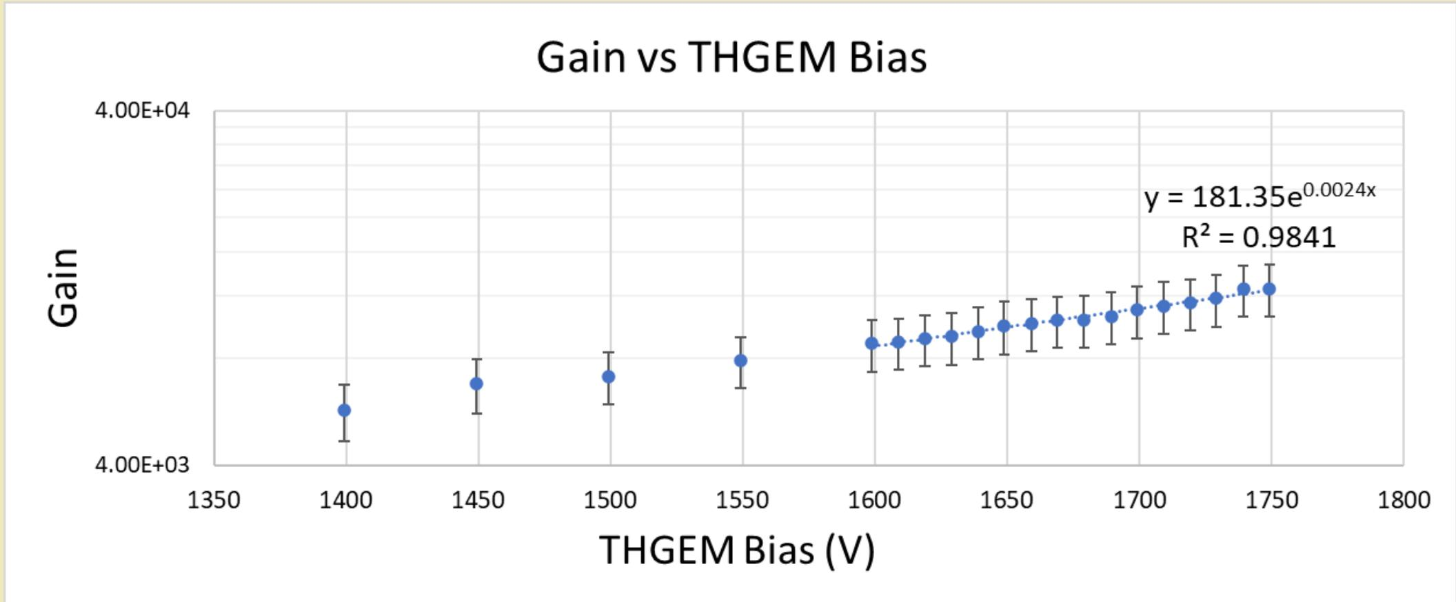
Incident Rate of  $1879.41 \pm 289.23$  based on Geiger counter values used. Max of 1750V to avoid discharges typical beyond 1800V.
