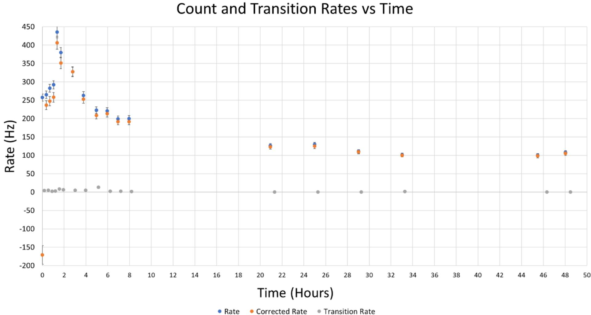
Notice the difference between Rate and Corrected shrinks over time, meaning negative pulse (and overshoot) rate drops over time
