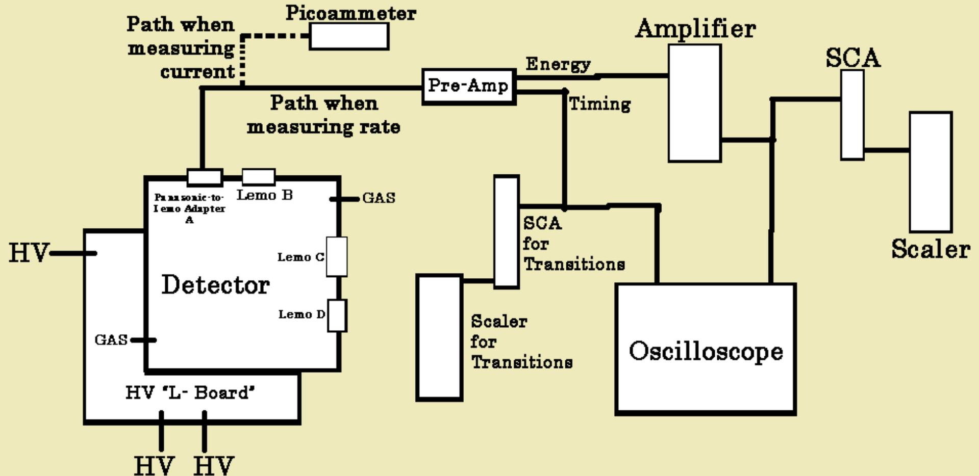
Readout electronics chain used during testing. Note: Energy and Timing outputs from the Pre-amp are just labels; the signal out of both is identical. SCA: Single Channel Analyzer.
