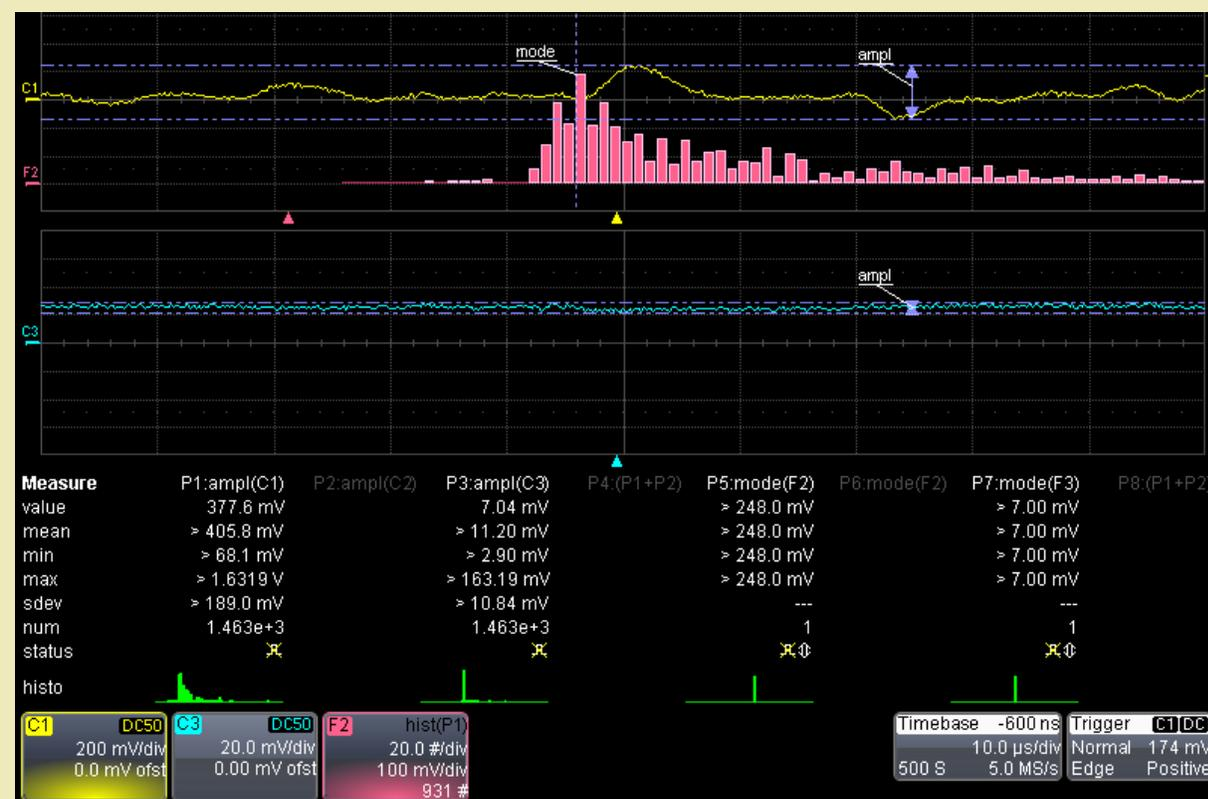
Histogram with amp signal at beginning (left) and end (right) of 48-hour study, negative polarity
