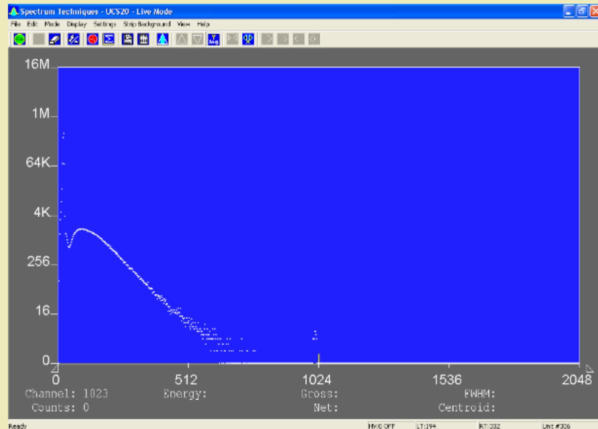
Initial pulse-height measurements taken using a Multi-Channel Analyzer source-off (left) and source-on (right)
