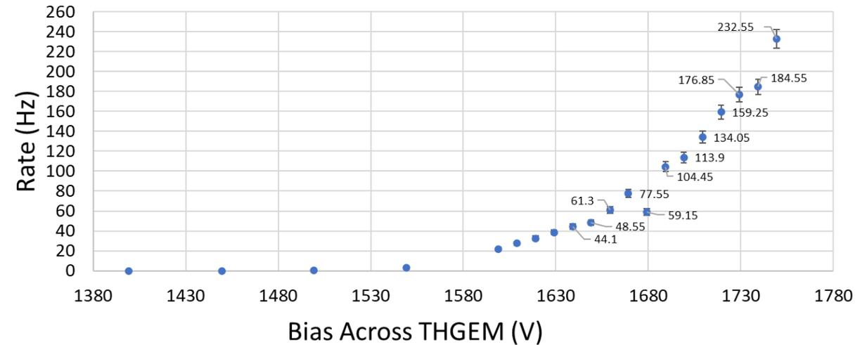
Rate increases due to increase in field in the holes
