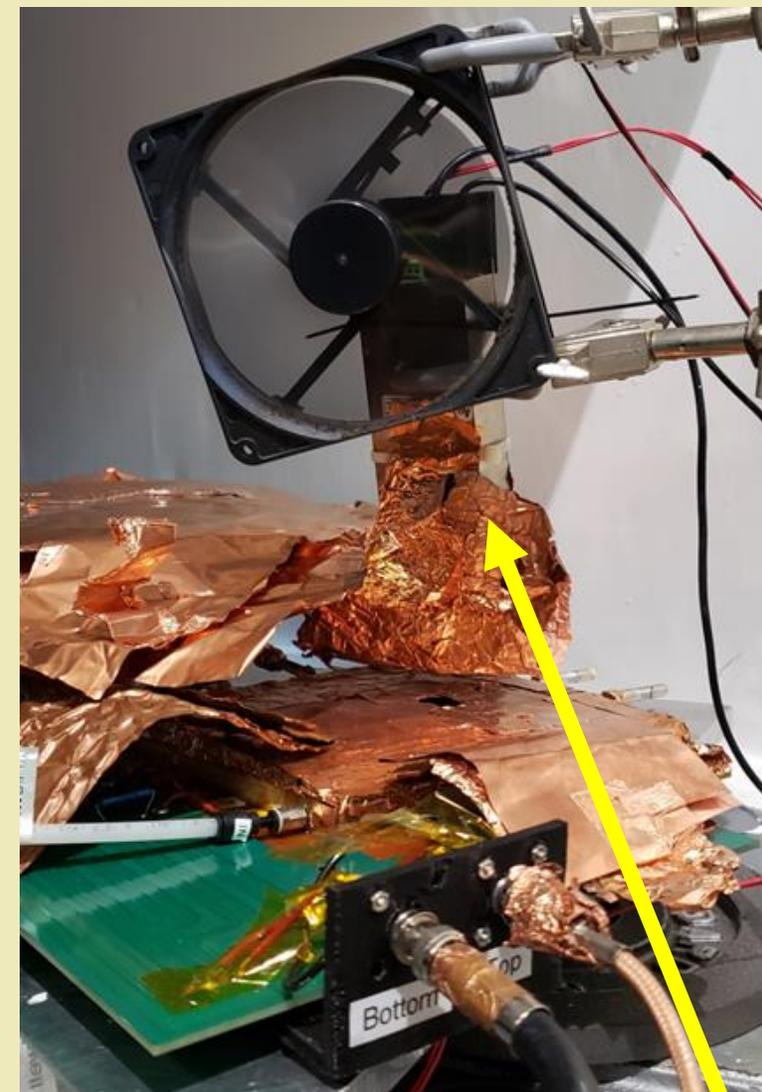
Arrow indicates the X-ray gun. The purpose of the fan is to keep the X-ray gun cool and maintain operating temperature
