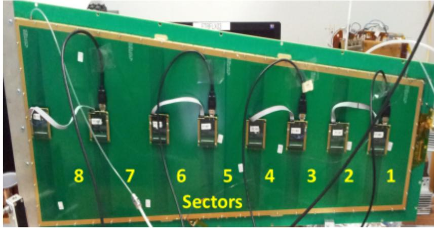
Figure 3.27: A large-area GEM detector with radial zigzag strips read out with eight APV hybrids connected to eight  $\eta$ -sectors through Panasonic connectors.
