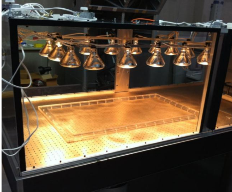
Figure 2.8: Completed 1 m 50 cm light rack and empty stretching frame [17].
