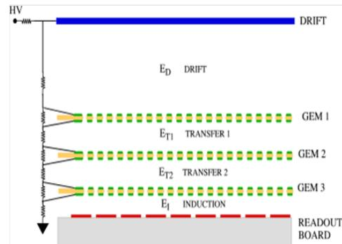
Fig. 2. Triple GEM Geometry
