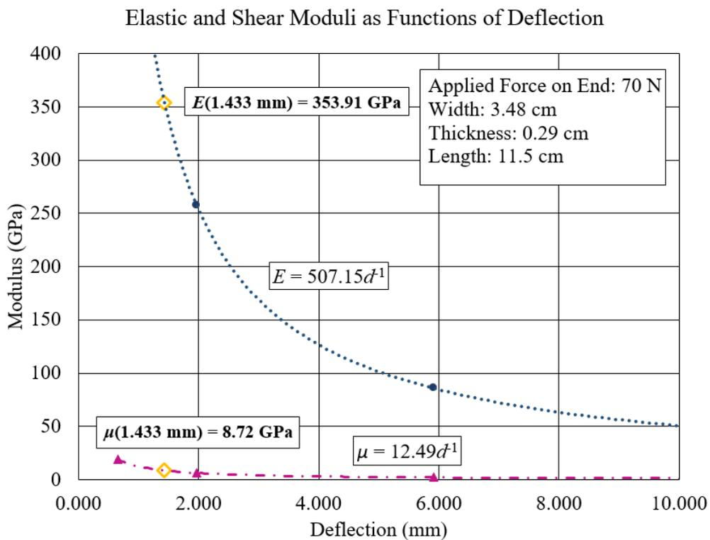
Figure 8: The Young's (elastic) and Shear moduli as functions of deflection; the yellow diamonds show the moduli of the IM7/090 with Araldite composite.
