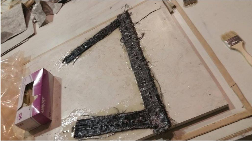
Figure 4: The laminated partial frame shown on the mold.
