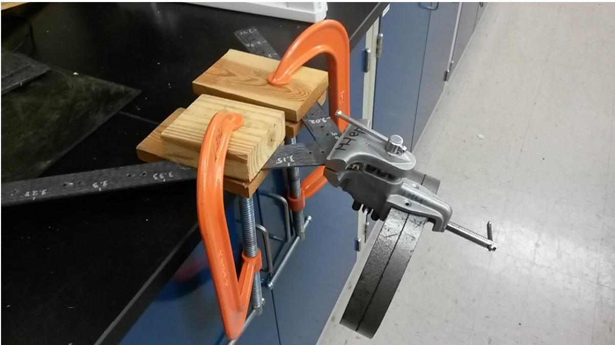
Figure 5: Testing the corners of the partial frame by hanging weights ranging from 4.9 to 10.5 kilograms on the corners; shown are 10.5 kilos hanging on the “butting” corner.
