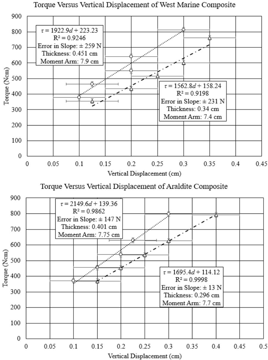
Figure 3: Comparison of West Marine and Araldite carbon fiber composites.
