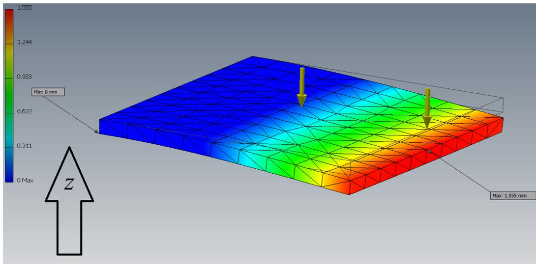
Figure 2: Simulation of Araldite test plate deflecting due to a 7.1 kilogram weight hanging on the end of the plate.
