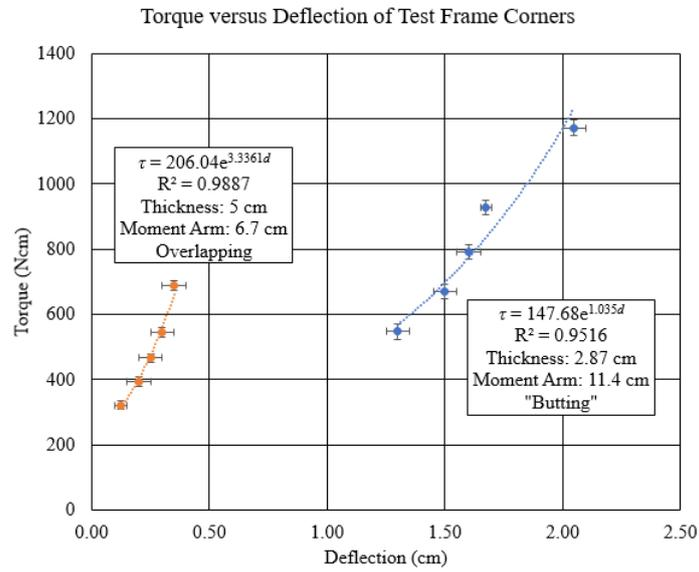
Figure 6: Torque exerted on the corners of the partial frames as a function of deflection.
