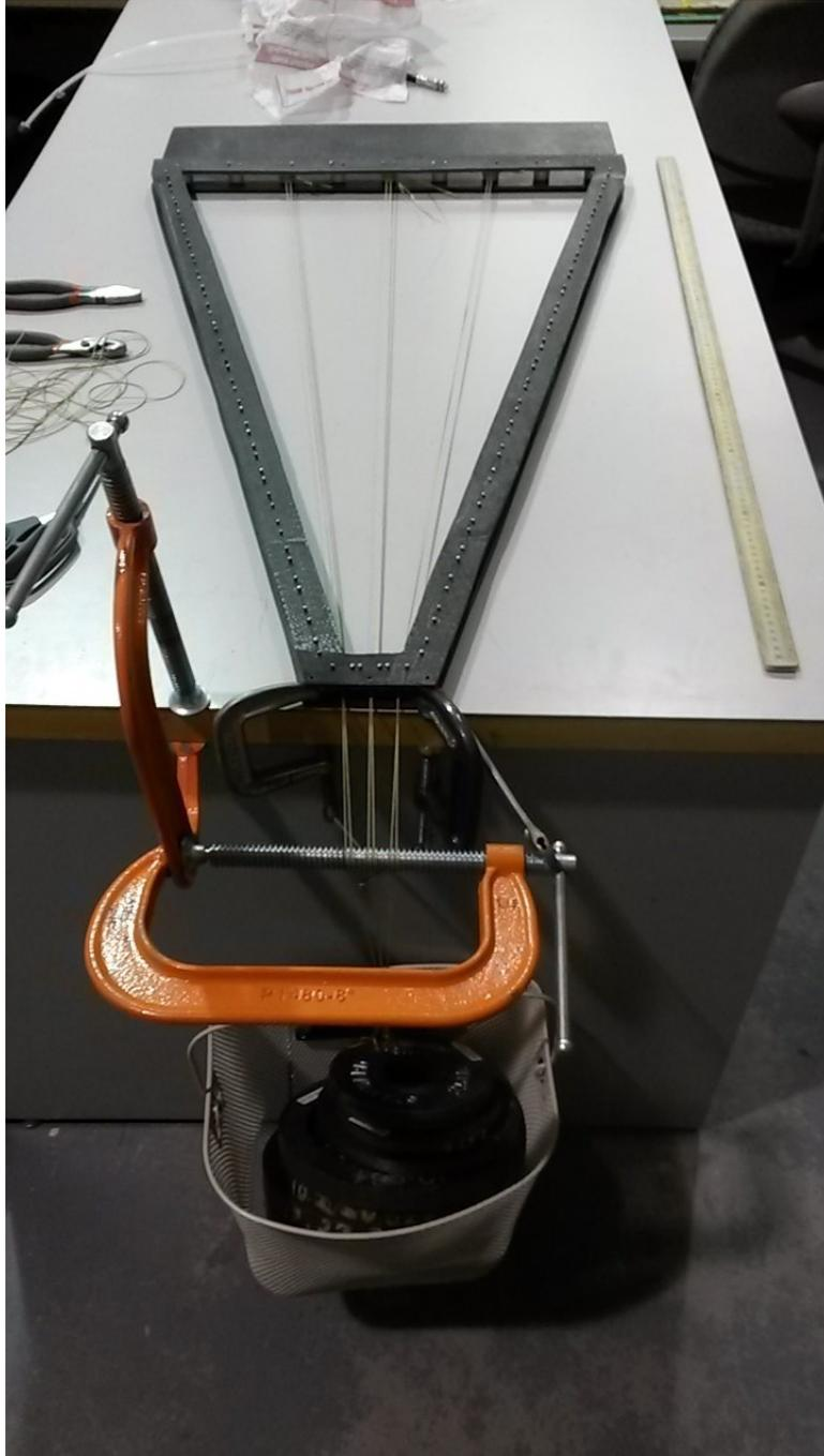
Figure 9: Setup of the full frame experiment using three pairs of lines to translate tension; shown in the basket is 28.2 kilograms.
