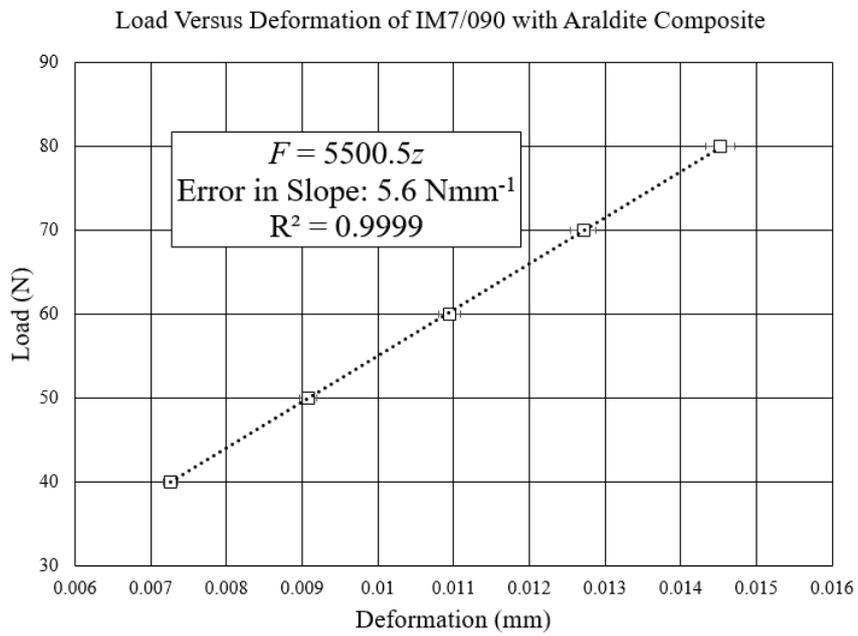
Figure 10: Applied force on the pullouts as a function of deformation in the  $z$  direction.
