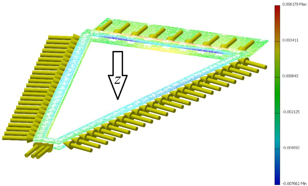
Figure 7: A simulation of the full carbon fiber frames in the  $z$  direction with 70 Newtons applied on each pullout part, emulating the foil assembly (units are millimeters); as can be noticed, the deformation in the corners is negligible compared with the sides.
