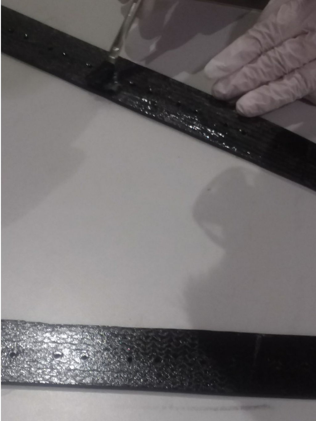
Figure 6: Applying glue on the support frame using a brush
