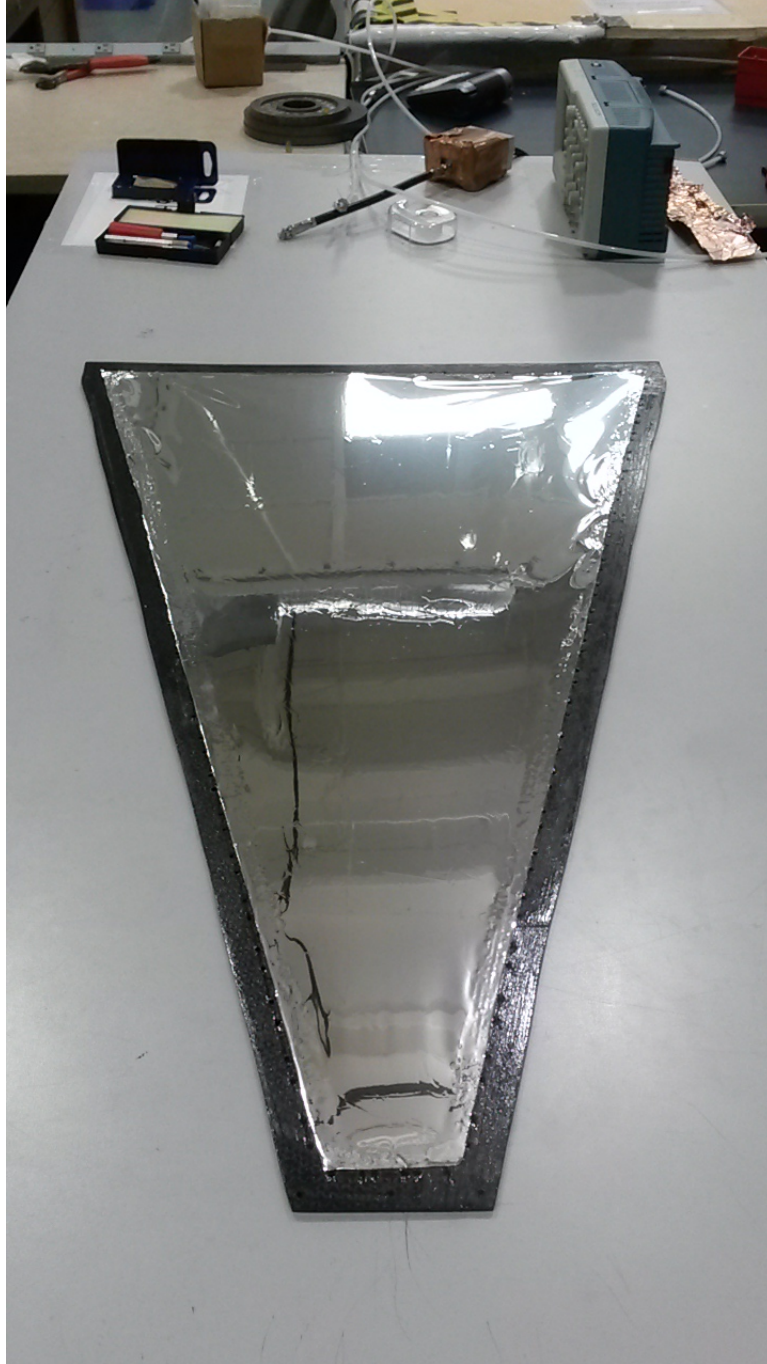
Figure 9: Al KAPTON foil on drift frame, view of how finalized job should look
