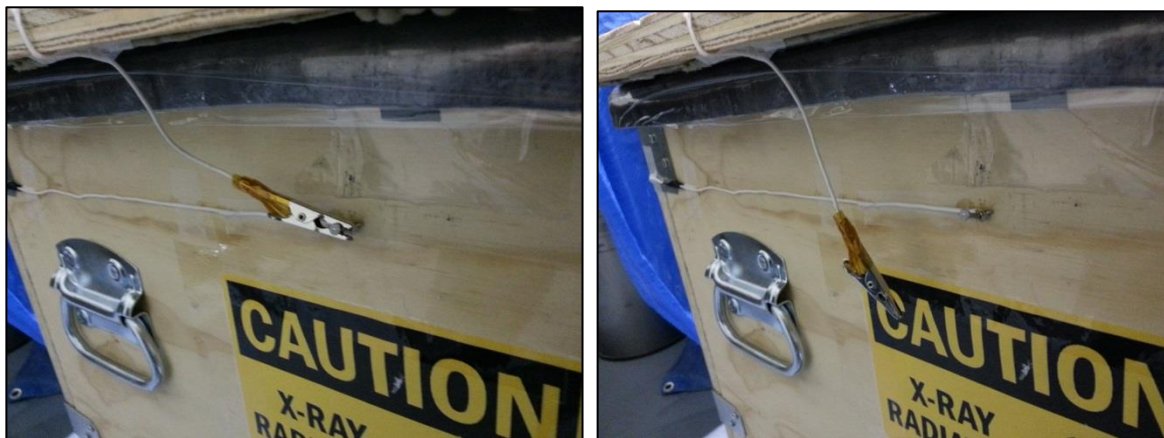
Figure 18: Completed expanded box with Interlock wires now installed (left=on, right=off)
