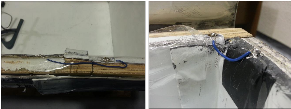
Figure 18: Completed expanded box with Interlock wires now installed (left=on, right=off)
