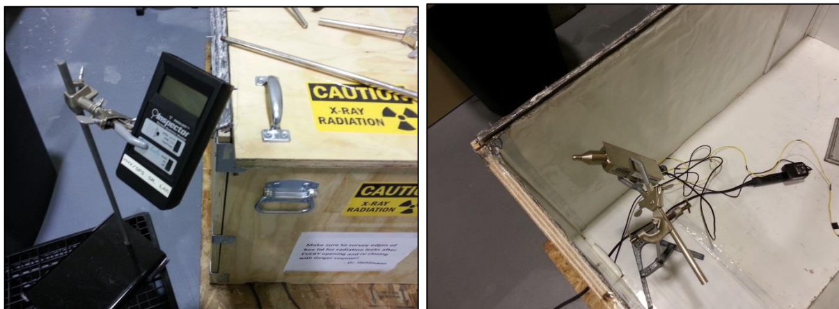
Figure 21: Radiation leak testing setup
