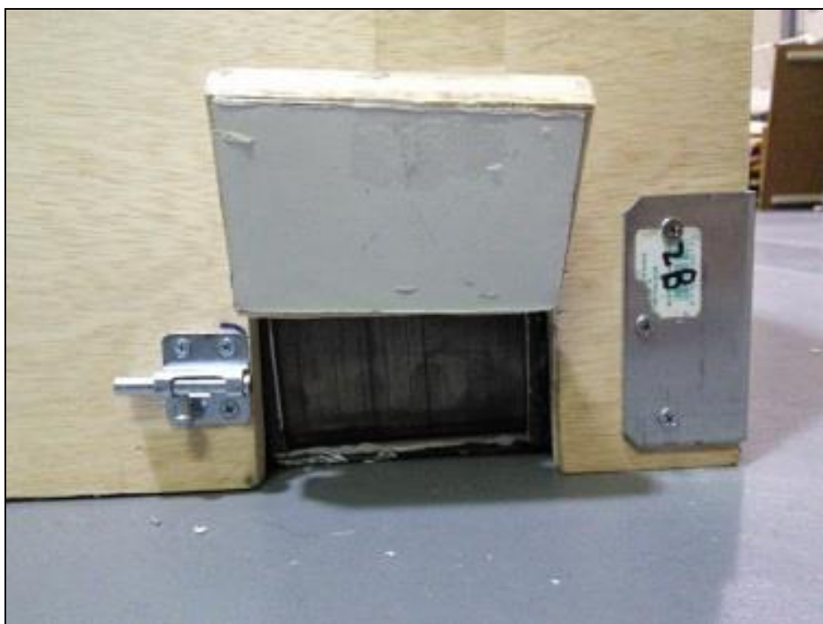
Figure 12: Outside view of access port #2 in its open position. The back of the Velcro-attached solid seal from Fig. 10, as well as the inside lips of the 'picture frame' seam-sealer, are shown too. Notice the inside of the hinged wood piece is also covered in its own lead paneling.
