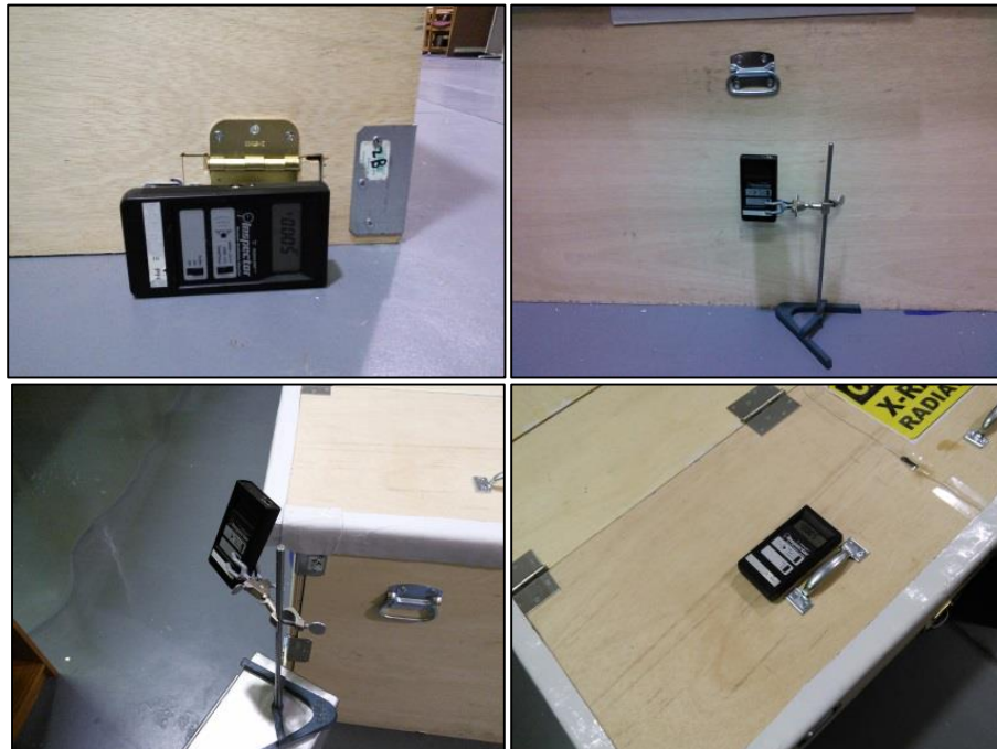
Figure 28: Examples of the Geiger counter in some actual testing positions. (Top Left) Access Port #2; position number 2. (Top Right) Side Panel Clean Mid; position number 24. (Bottom Left) Corner Clean-Parking Top; position number 17. (Bottom Right) Lid Panel Parking; position number 31.
