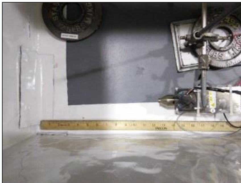
Figure 32: The Mini-X in its point blank testing position for Access Port #2.
