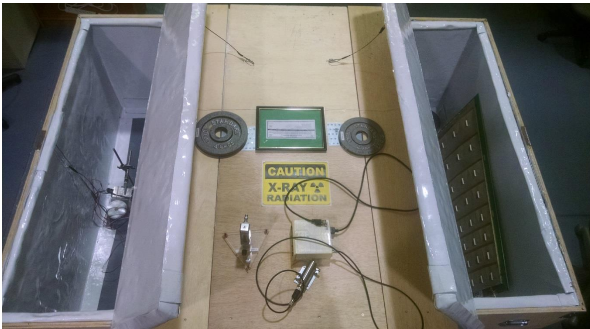
Figure 21: A final overview of the box with x-ray source and detector in respective testing locations.
