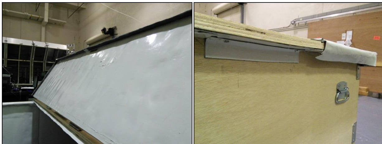
Figure 7: Close-ups of exterior top-edge seals on and round the lid doors. These seals were added as response to radiation leaking from separation between the lid and tops of the sides of the LLB.
