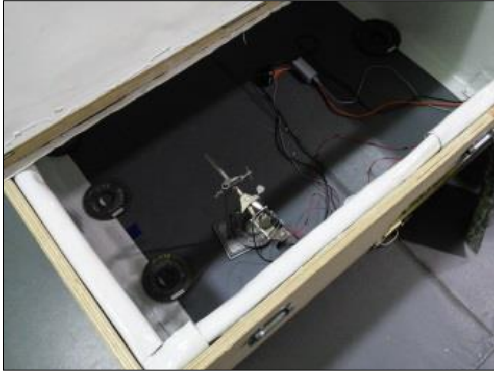
Figure 35: The Mini-X positioned to fire straight up at the lid for a point blank test.
