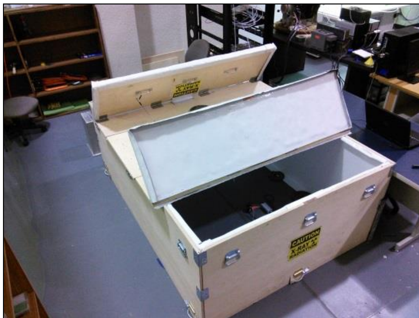
Figure 5: The LLB with both lid doors open. Each lid weighs around 50 lbs. and has a metal kickstand to hold it open and safety cables to prevent it from slamming shut.
