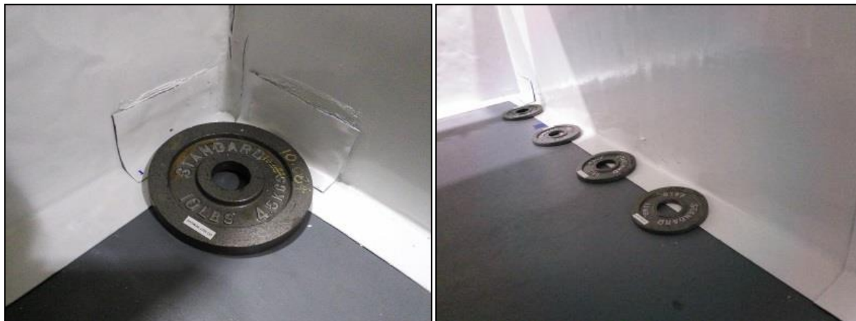
Figure 17: Various 5 lb. and 10 lb. weights used to reduce leaks on the inside of the box.
