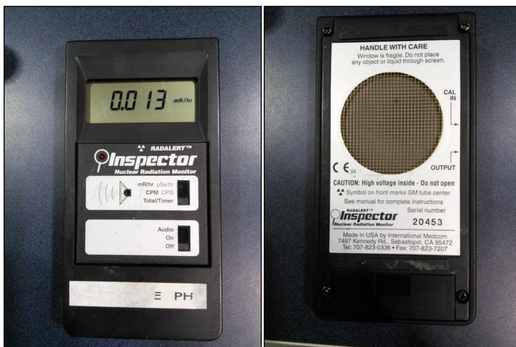
Figure 1: Radalert Inspector Nuclear Radiation Monitor. (Left) The measurement/settings readout side. The Audio/On/Off switch was set to 'Audio' for all safety checks and regular testing. (Right) The detector-side.
