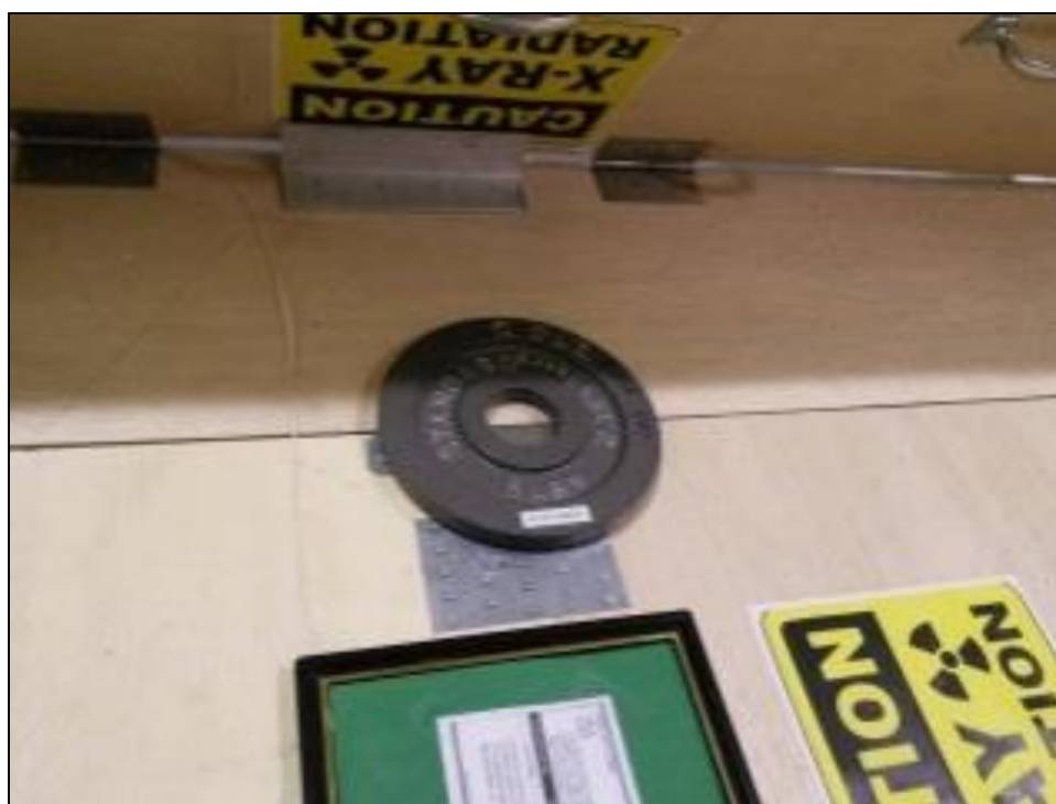
Figure 18: Additional weight (1 of 2) on the lid of the box to reduce separation between pressed lead sheets and thus stop radiation leaks.
