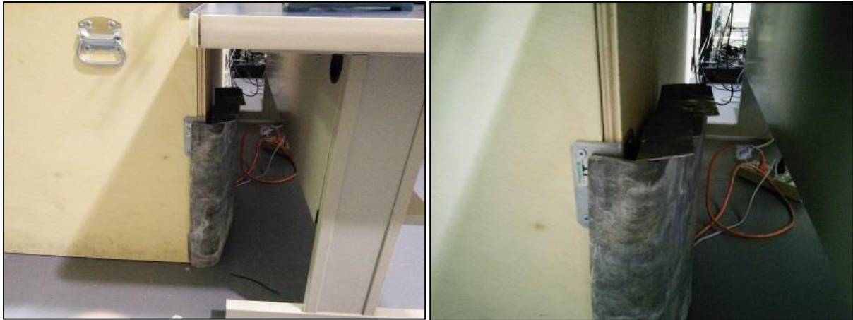
Figure 15: Different views of the external shielding including the 3 pieces of 1/16 in. thick lead sheet placed on top of the 0.25 in. thick sheet.
