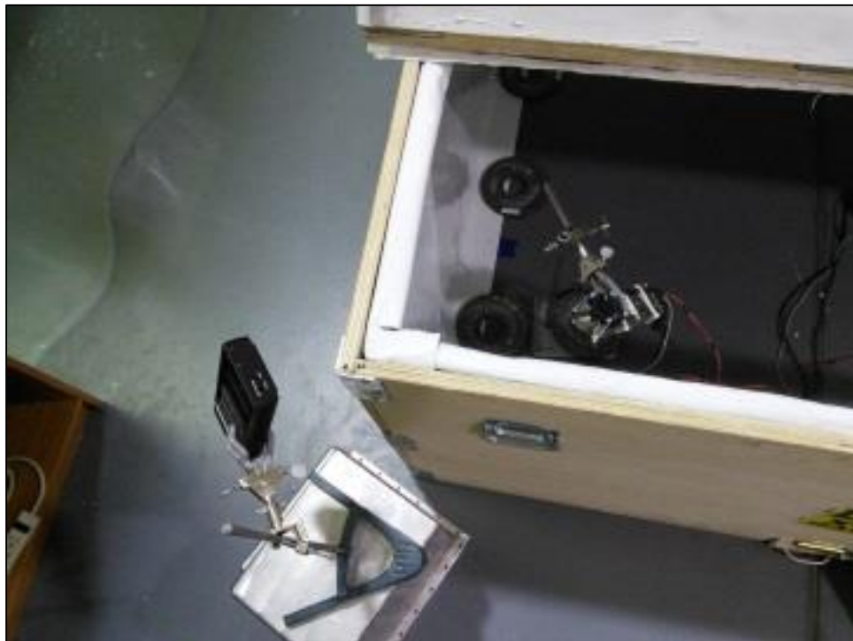
Figure 34: A view of both the Geiger counter and the Mini-X positioned to point-blank-test a top corner.
