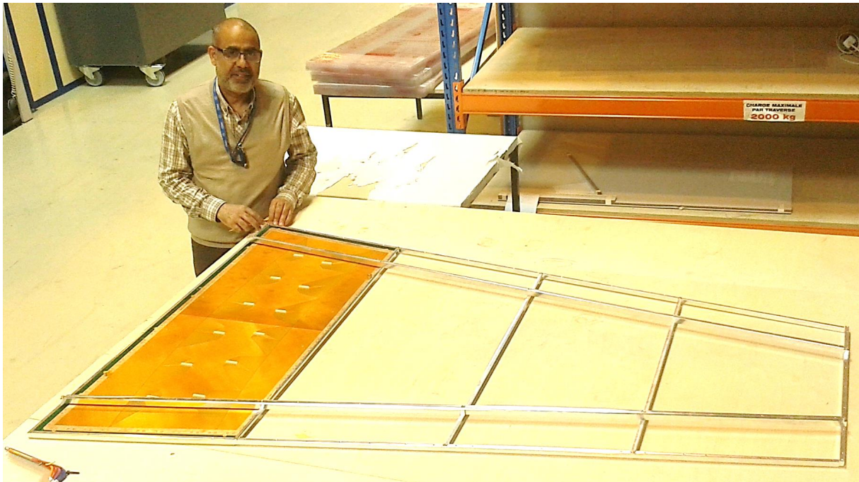
Figure 6.38: Prototype of GE2/1 aluminum coupling frame; the M4 prototype module is fixed on the structure in its final position.
