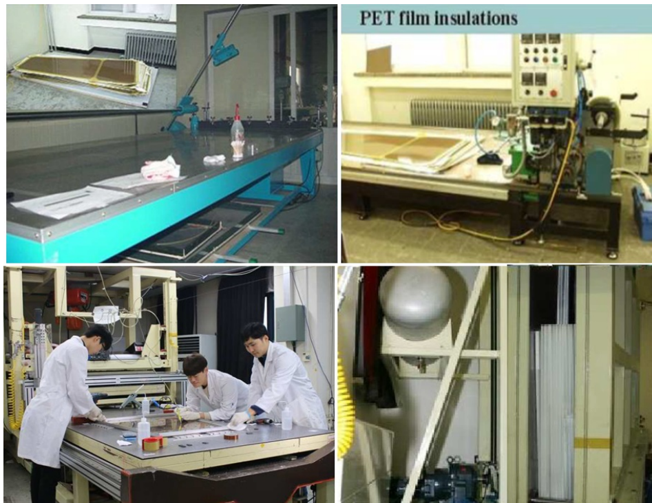
Figure 5.22: iRPC production: a silk-screen table for the graphite coating (top left), a device for the PET insulation (top right), optical tables and multi-layered air-pressing tubes for the composition of gas gaps (bottom left), and oil tanks and a pressing device for the oiling procedure (bottom right).
