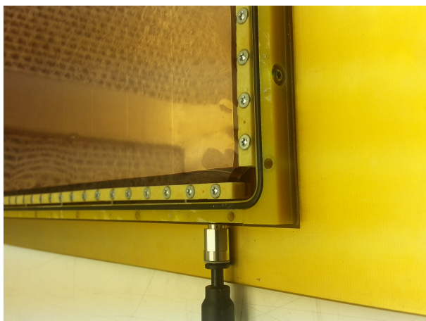
Figure 14: Wrinkled corners on a stretched GEM foil
