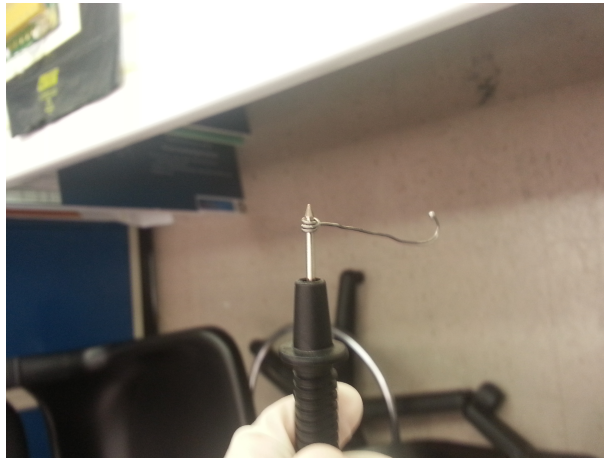
Figure 12: Small probe to test for electrical connection between foils and springs
