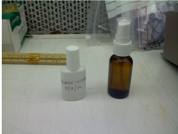
Figure 5: Threebond cyanoacrylate glues. The white container is the glue, while the brown container is an accelerator.
