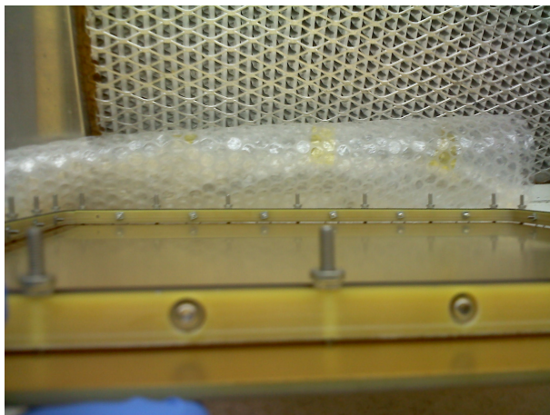
Figure 3: The gap that you should leave between your frame sides and the drift board
