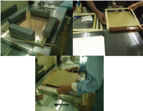
Fig. 6. GEM stack glued with weight (left); taking out the alignment frames (right); gluing the GEM stack onto the readout plane (bottom).
