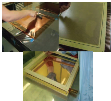
Fig. 4. Gluing the Kapton side of the drift (left); undesirable air bubble after gluing the drift cathode and honeycomb plate (right); gluing the drift cathode spacer (bottom).
