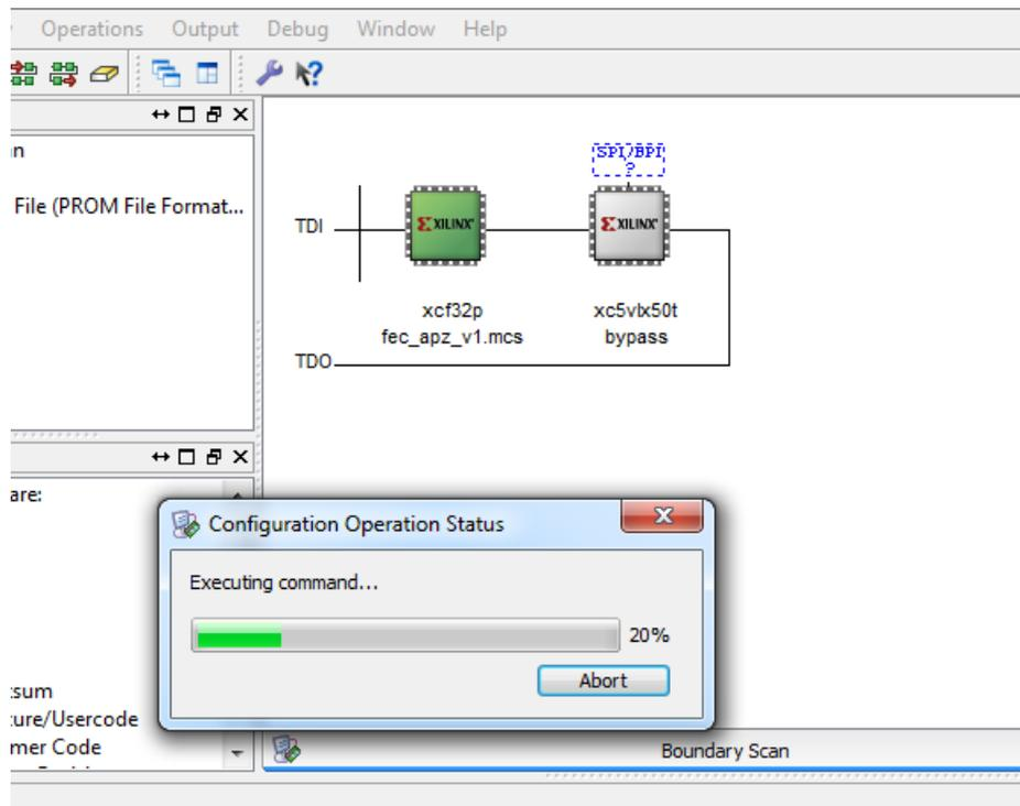
e) If the programming procedure was successful Impact will display "Program Succeeded". You can now power cycle the FEC board to load the new firmware from the boot EEPROM.
