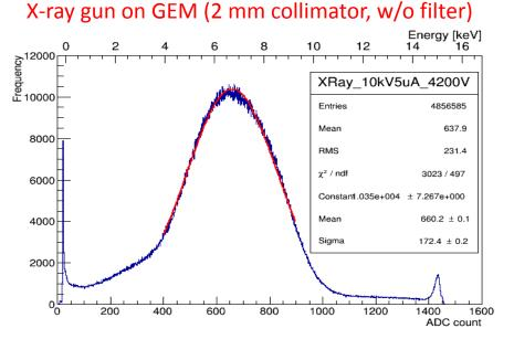
Calibrated with Fe-55, X ray energy is <u>7.39 keV</u> @ 10kV/5uA settings.
