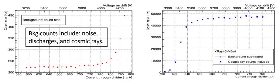
Peak shifts to right when increasing HV on GEM as gain increases
