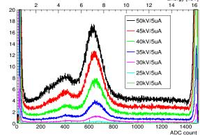
X ray spectrum at 5 uA, distance 45 cm,  $V_{drift}$  = 3980 V, I=734.5 uA, 2× 10<sup>4</sup>
