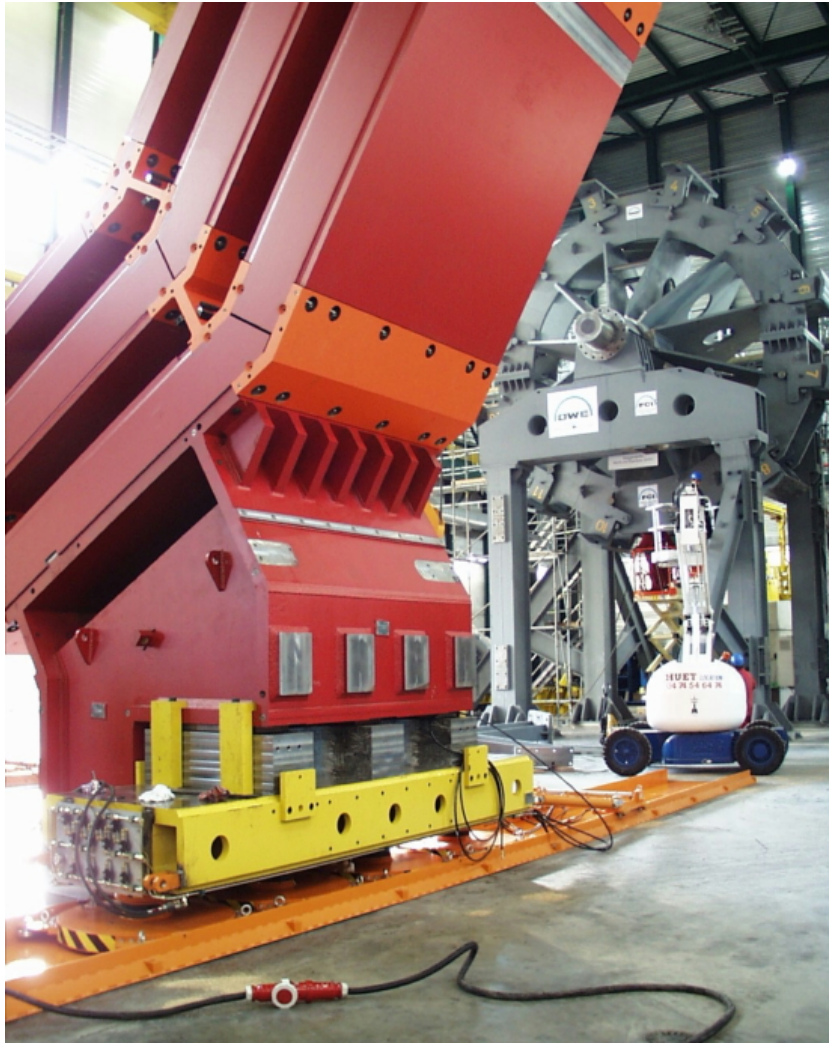
Figure 248: A transport beam for barrel rings with 4 air pads fixed on it.
