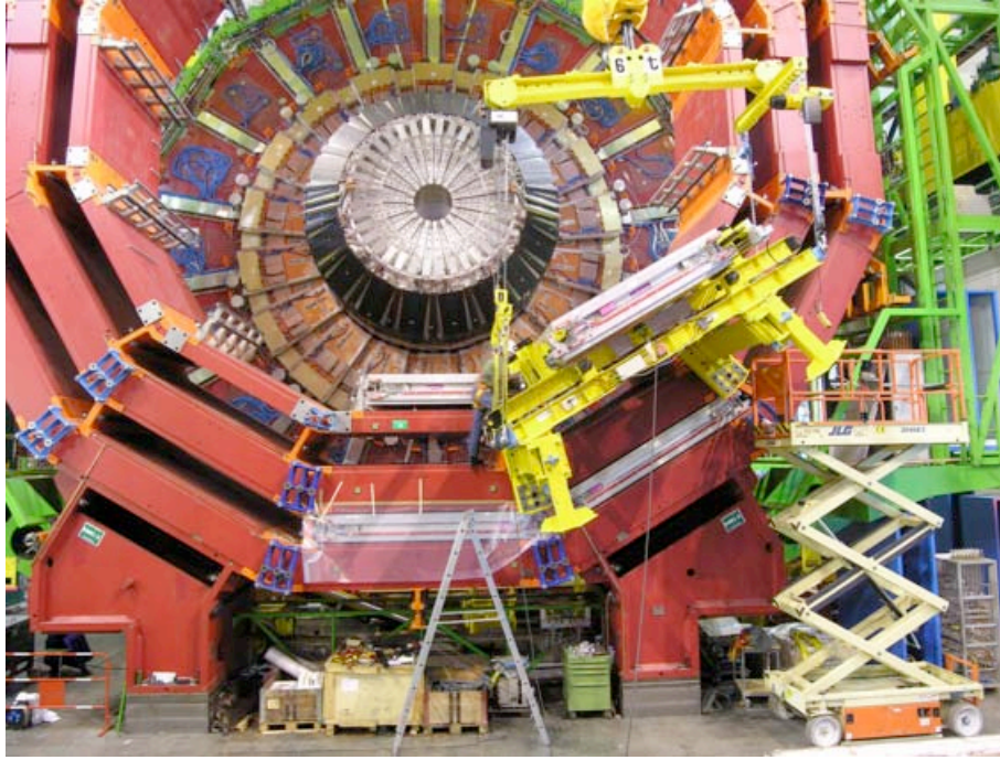
Figure 154: Installation of MB1 station on Wheel -2. The yellow frame is the cradle used to insert the chamber in its location inside the iron slot.
