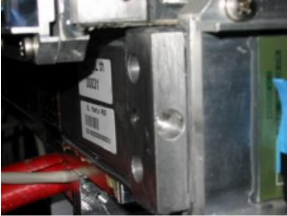
Figure 139: Corner blocks of an SL. These pieces also carry the reference marks with respect to which the wire positions are measured.
