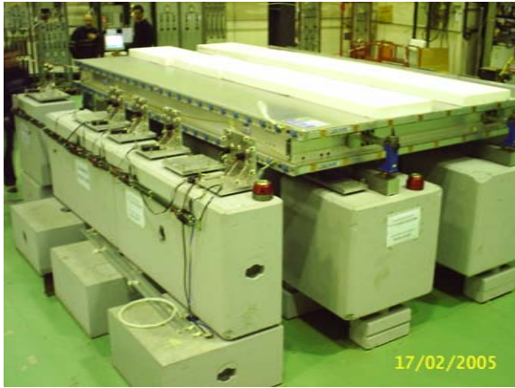
Figure 152: The chamber calibration bench in the CERN ISR Lab.
