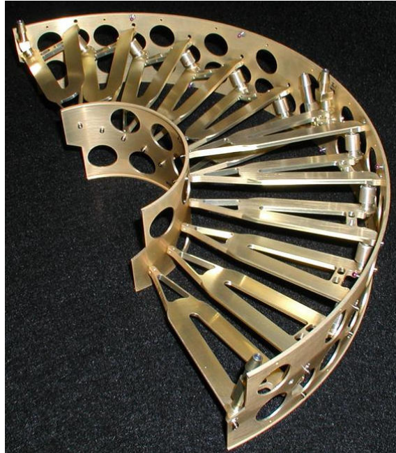
Figure 44: The FPix half-disk cooling channels mounted in the outer half-ring structure. The turbine-like geometry is apparent. Panels are mounted on both sides of the cooling channels.
