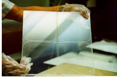
Figure 111: View of a typical tile of HO with WLS fibres inserted in the 4 grooves of the tile.
