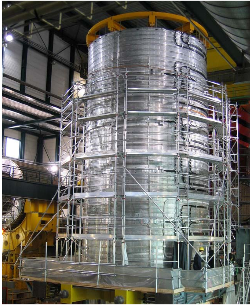
Figure 6: The cold mass mounted vertically before integration with thermal shields and insertion in the vacuum chamber.
