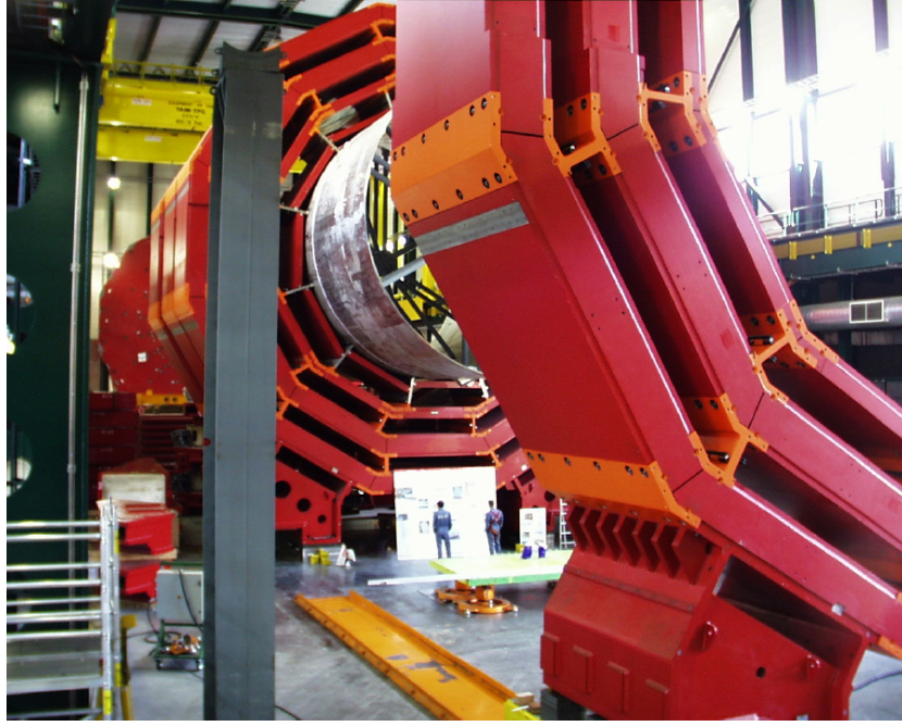
Figure 10: A view of the yoke at an early stage of magnet assembly at SX5. The central barrel supports the vacuum chamber of the superconducting coil. At the rear, one of the closing end cap disks is visible.
