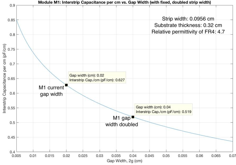
Figure 6: Interstrip capacitance per cm of strip length vs. gap width, with doubled, fixed strip width for Module M1.
