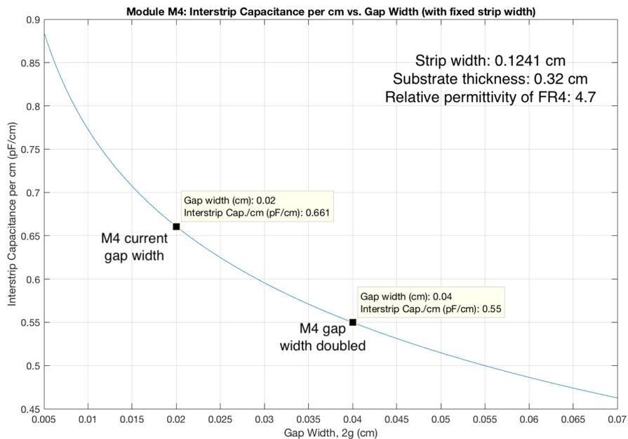
Figure 3: Interstrip capacitance per cm of strip length vs. gap width, with fixed strip width for Module M4.
