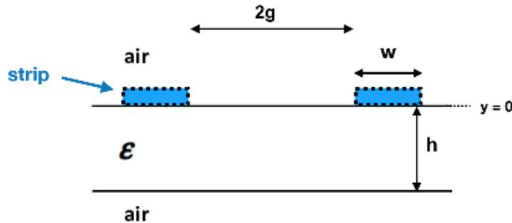
Figure 1: The strip geometry, where  $w$  is the strip width,  $2g$  is the gap width, and  $h$  is the thickness of the substrate with dielectric constant  $\epsilon$ .
