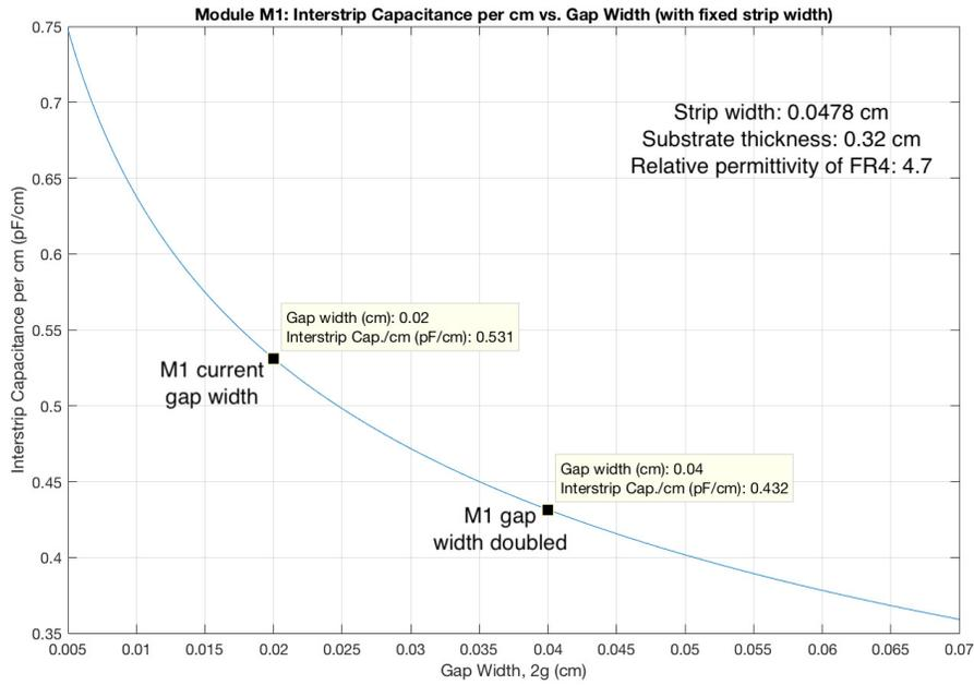
Figure 4: Interstrip capacitance per cm of strip length vs. gap width, with fixed strip width for Module M1.
