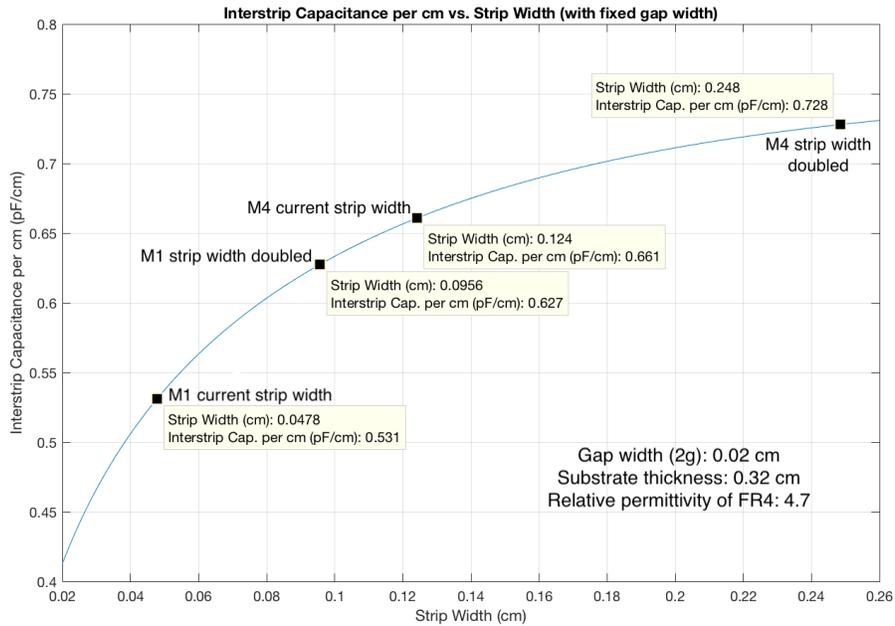
Figure 2: Interstrip capacitance per cm of strip length vs. strip width, with fixed (current) gap width.
