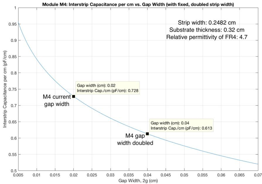
Figure 5: Interstrip capacitance per cm of strip length vs. gap width, with doubled, fixed strip width for Module M4.
