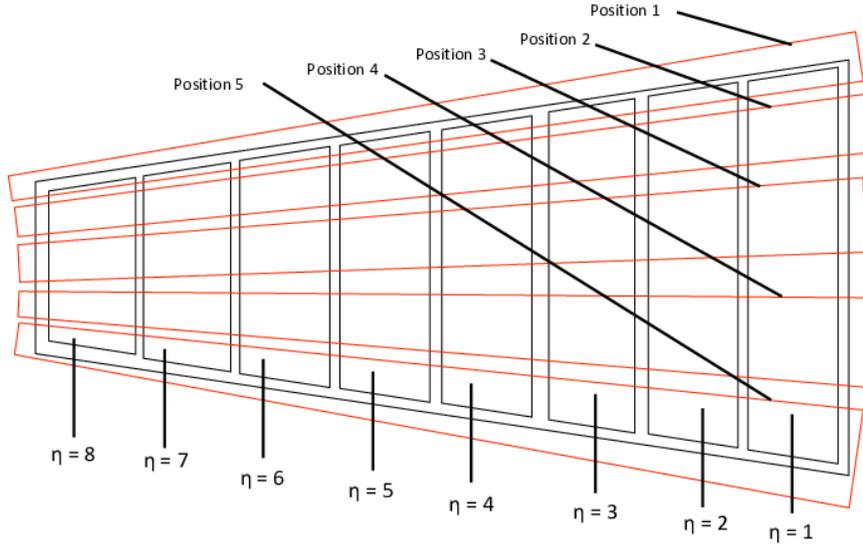
Figure 7: Location of the positions where measurements were taken in each eta sector on the GE1/1-X-S RO.
