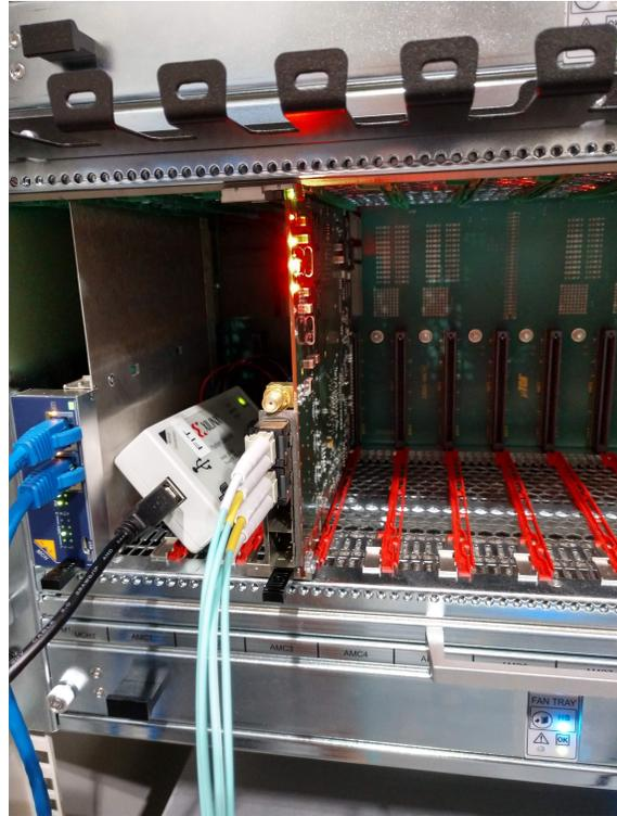
(b) GLIB card with the bottom tab pushed in. Note the illuminated green LED and the red LEDs at the top.
