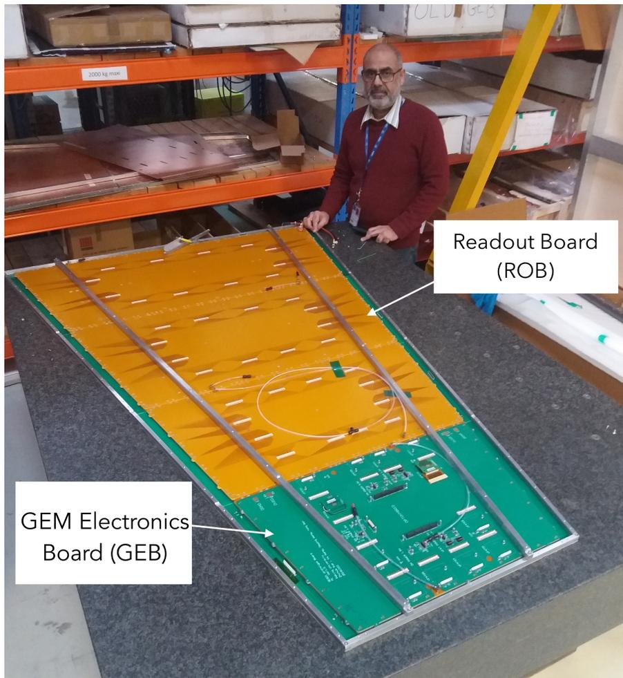
Figure 3: A photo of the first fully assembled GE2/1 chamber [2]. Note the un-instrumented GEB board fixed to the M1 (smallest) module of this GE2/1 back chamber.
