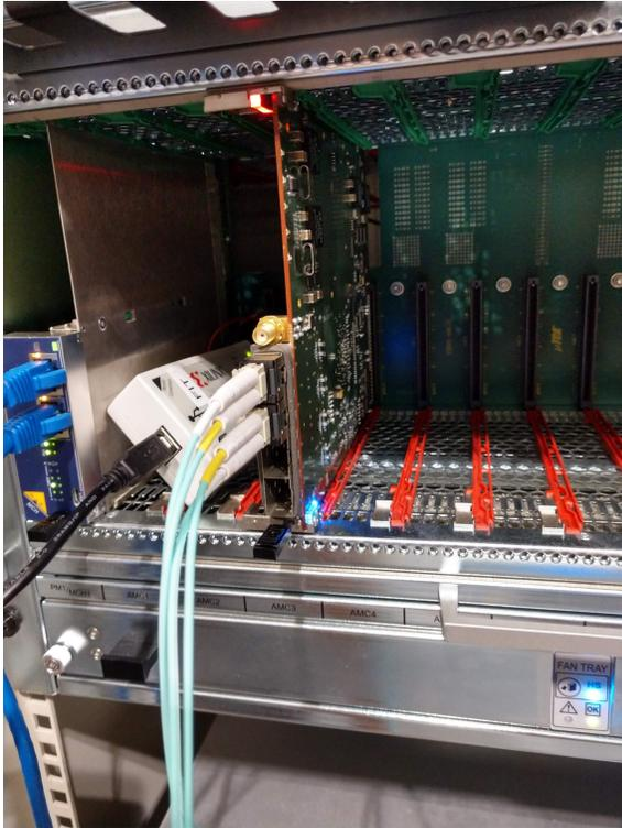
(a) GLIB card with the bottom tab pulled out. Note the illuminated blue LED at the bottom of the card.
