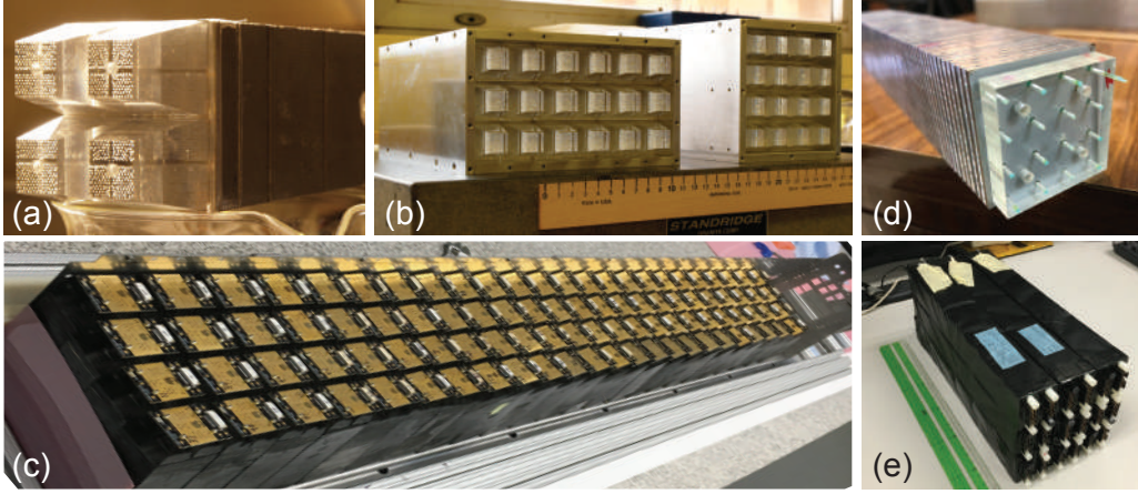
Figure 14.8: (a)-(b) W-SciFi calorimeter modules assembled during early stages of R&D. (c) Assembly of a complete sector of the sPHENIX calorimeter based on W-SciFi technology. (d) W/Shashlik calorimeter with 80% W and 20% Cu absorber plates between scintillating tiles read out with WLS fibers. (e) Assembly of 9 prototype W/Cu shashlik modules.
