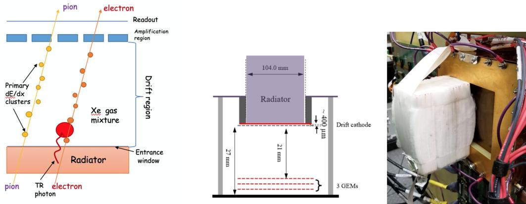
Figure 1: The basic concept of GEM-based TRD ( left), the prototype scheme (middle), and prototype at the testbeam setup (right)
