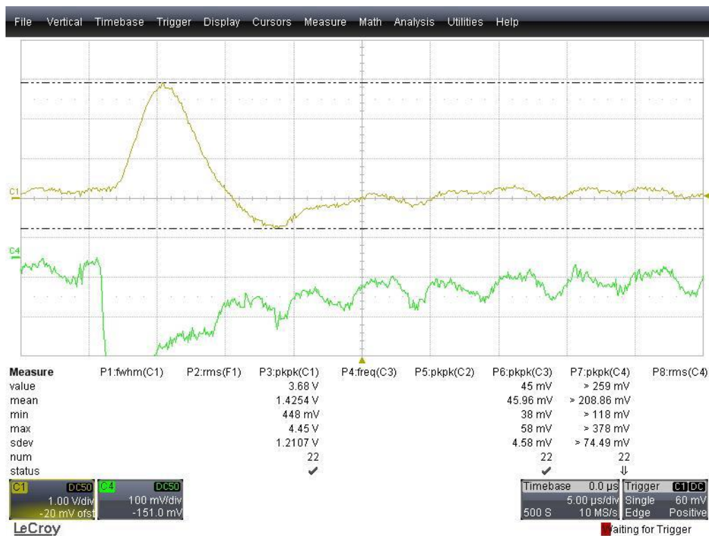
Figure 30. Oscilloscope Screenshot Cd-109 Source Detector Response. (C1) Signal from amplifier and preamplifier. (C4) Signal from preamplifier.
