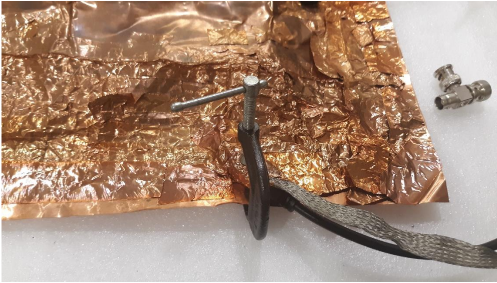
Figure 7. Image of Ground Strap Connection to GEM Bottom 3 Output
