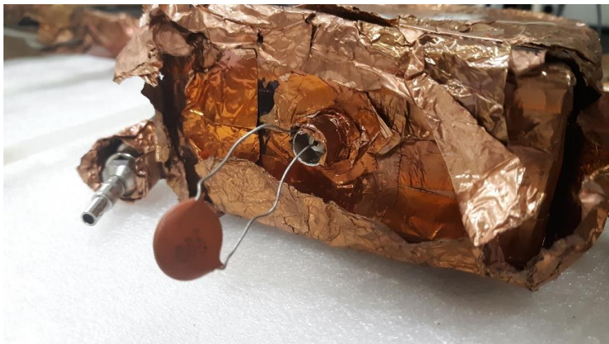
Figure 17. Capacitor Configuration on Preamplifier for Capacitor Test
