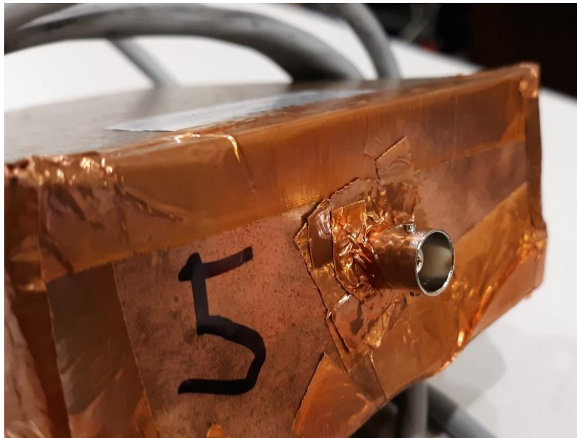
Figure 4. Copper Foil and Tape Shielding on Preamplifier 5 Input Port Plate
