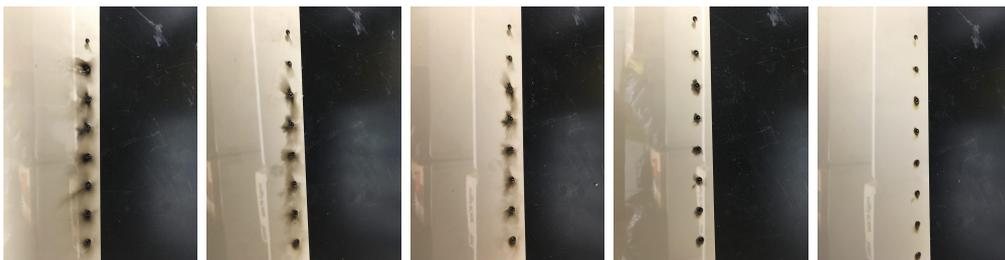
Figure 6: Cleaning of burn marks on PEEK plate; From left to right: original burn marks → clean with water → clean with 71% alcohol → clean with 91% alcohol → clean with acetone
