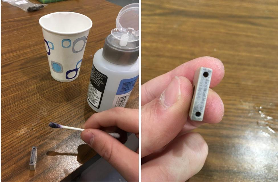
Figure 5: Cleaning of pull-out part with ink mark using acetone
