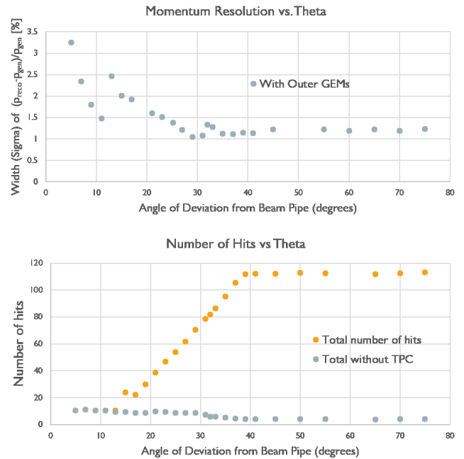
Fig. 10. Top: Momentum Resolution Uncertainty vs. Theta (test geometry). Bottom: Number of hits vs. Theta.
